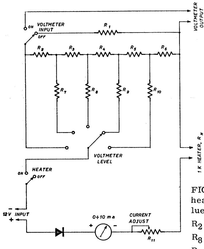
FIG. 3 - Circuit diagram of the heater supply. The resistor values are (in ohms):  $R_1 = 100$ ,  $R_2 = R_3 = R_4 = R_5 = R_6 = R_7 = 220$ ,  $R_8 = 470$ ,  $R_9 = 680$ ,  $R_{10} = 820$ ,  $R_{11} = 0 - 10000$ .
