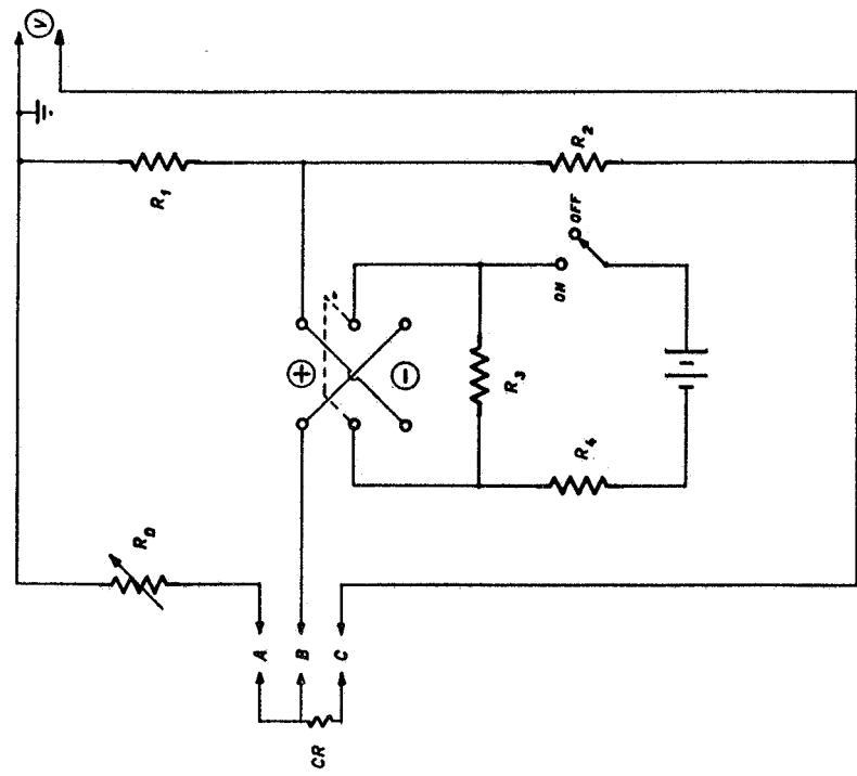
FIG. 2 - Circuit diagram of the bridge. The cell is a 1.36 v. mercury cell. The resistor values are (in ohms):  $R_1 = R_2 = 2000$ ,  $R_3 = 200$ ,  $R_4 = 10000$ .  $R_D$  is a standard resistor decade box.
