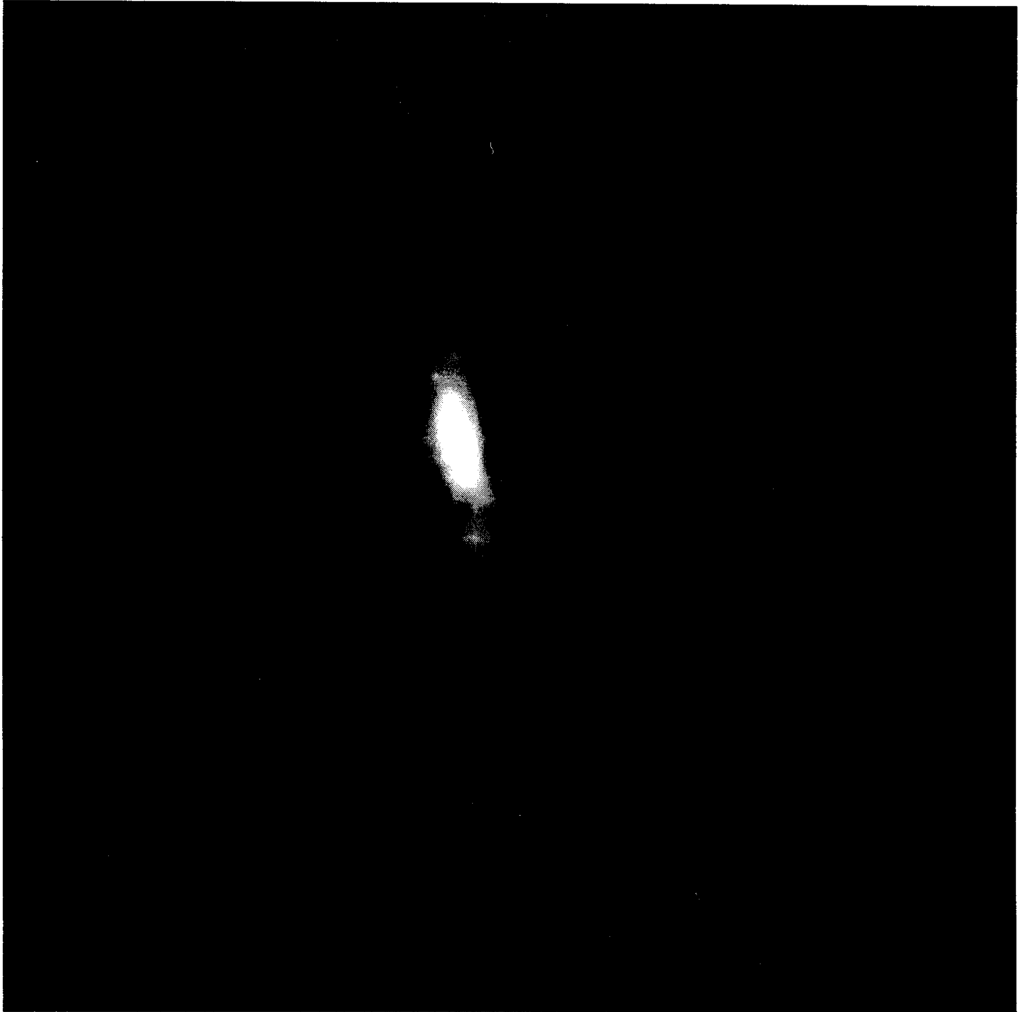
Figure 7: Beam image at 2 GeV. The scale of the figure is 100x100 pixels (in horizontal direction 1 px = 0.097 mm and in the vertical direction 1 px = 0.064 mm; the different ratios are due to the frame grabber acquisition).
