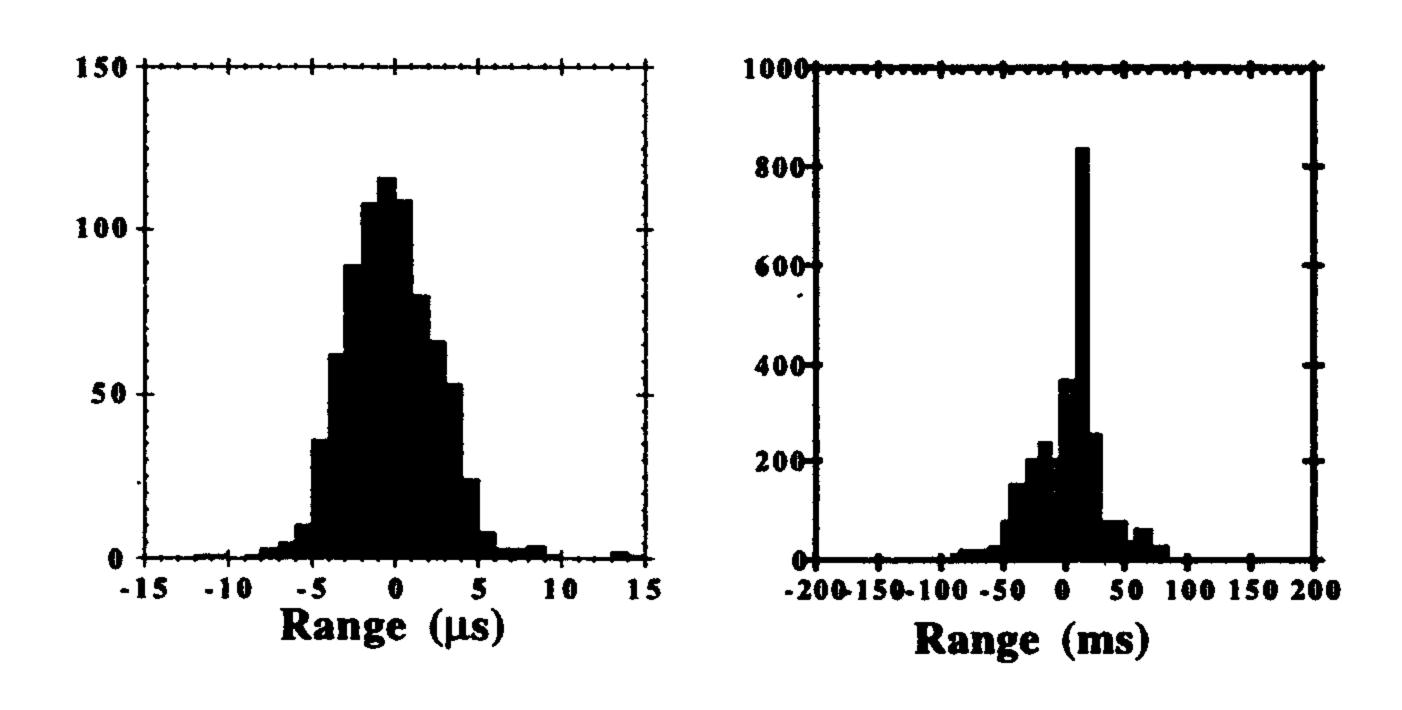
Fig 9. a) PPSs difference, b) Internal clock difference setted via ETHERNET
