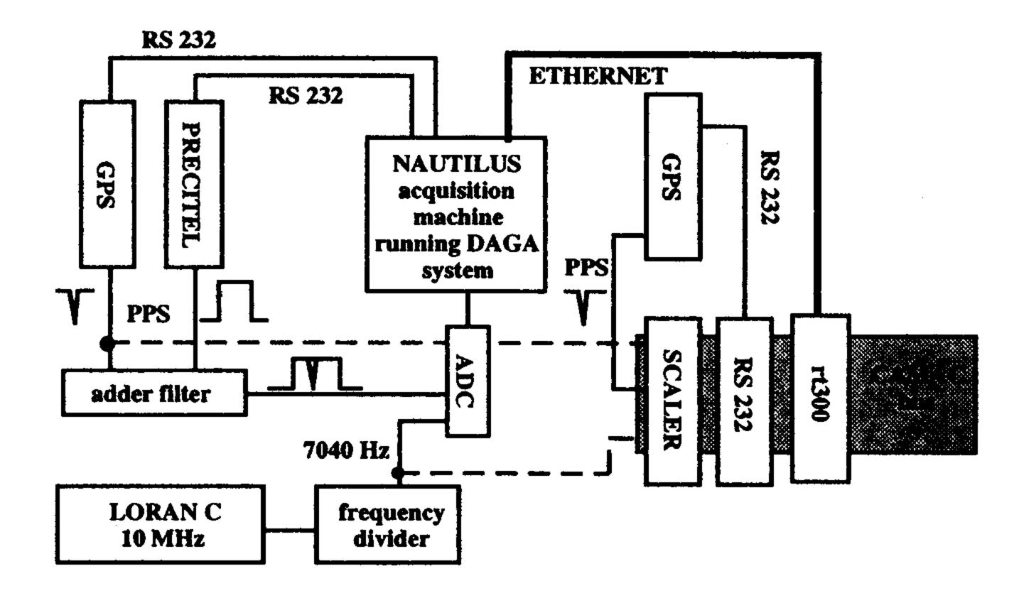
Fig 8. Timing system configuration
