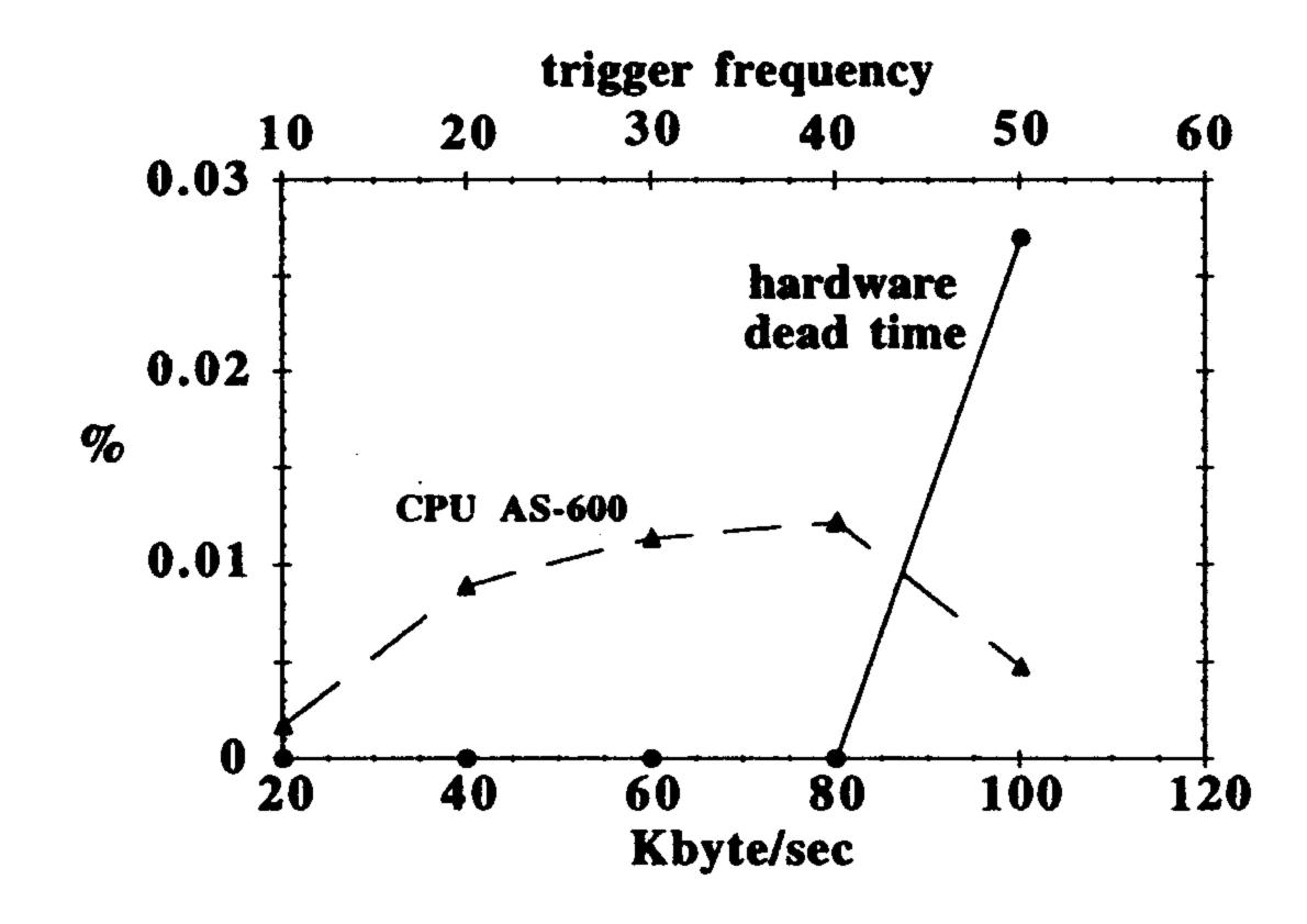
Fig 5. Percentage of dead time for VME system and remote CPU
