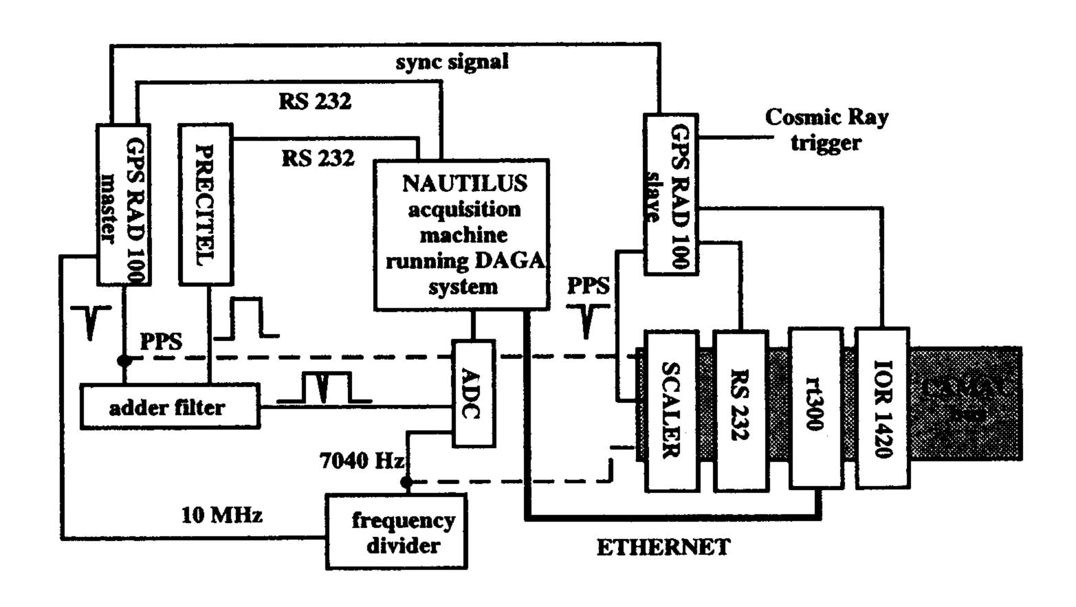
Fig 10. New timing system
