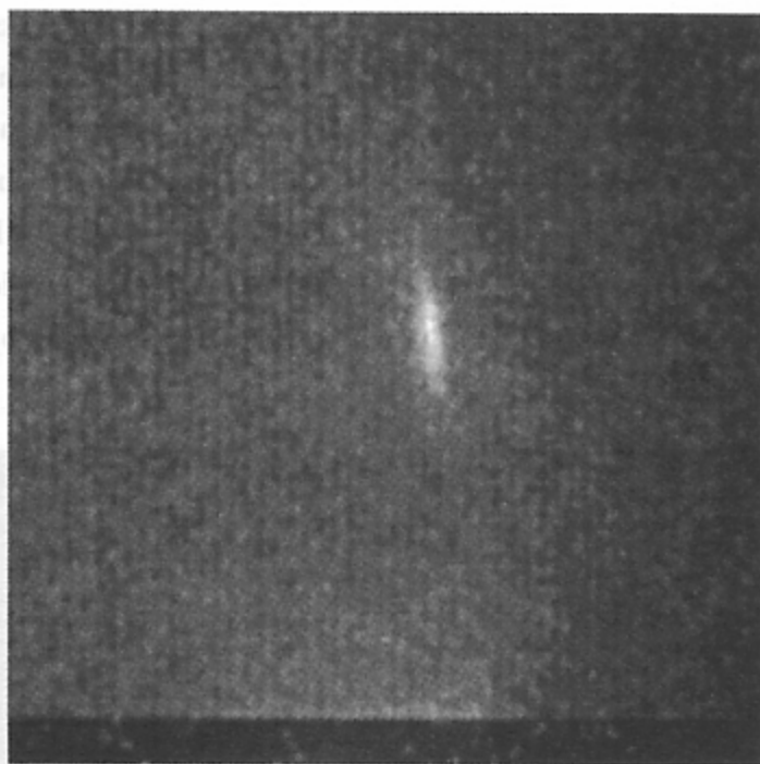
Fig. 9 - OTR image filtered by a horizontal polarimeter
