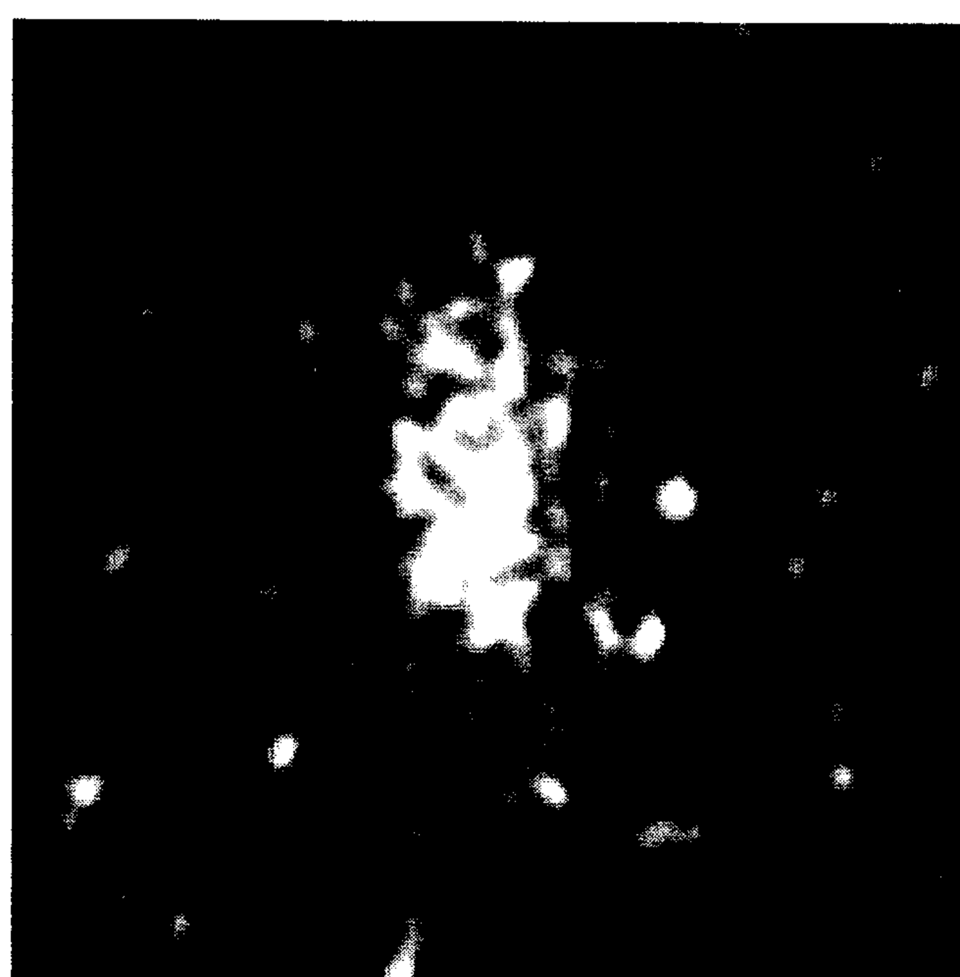
Fig. 1. Two OTR spots obtained with a 500 \mu A pulse 1 ms long at 1.1 MeV. The left picture shows a well focused beam; the right one shows a vertically defocused beam due to a current variation in the upstream quadrupole.
