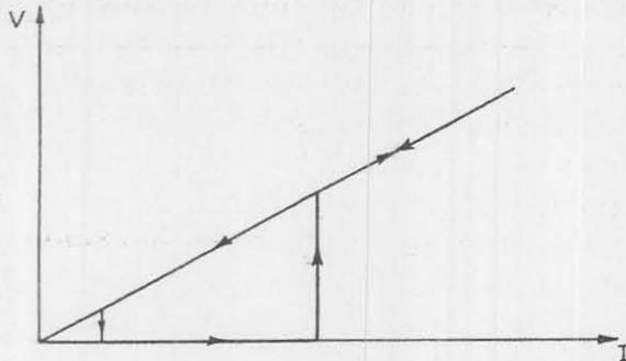
FIG. 3a - Current-voltage characteristics of a bare superconductor.
