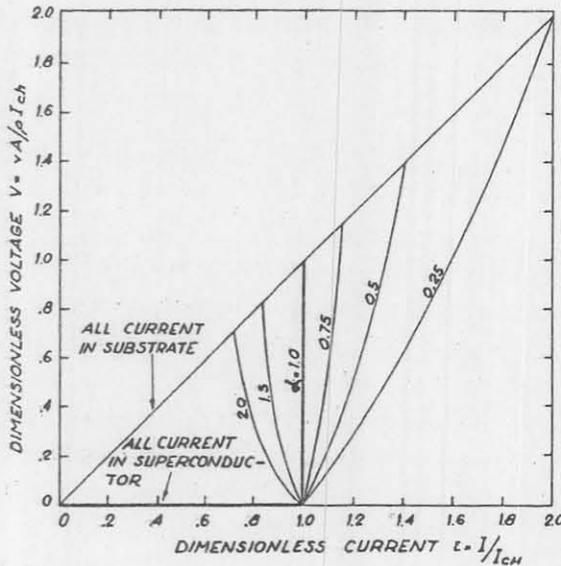
FIG. 4 - Current-voltage characteristic of a composite conductor for several values of  $\alpha$ .
