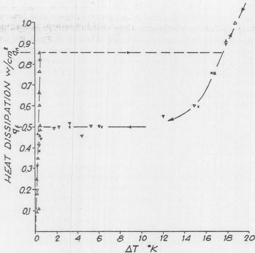
FIG. 2 - Heat transfer from a cable to liquid helium
