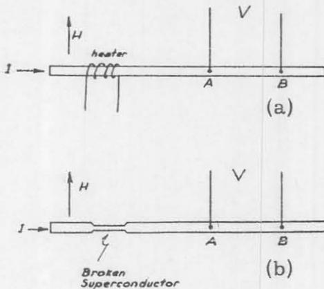
FIG. 6 - The heat-pulse method (a) and the broken-superconductor method (b) to obtain the minimum-propagating-current.
