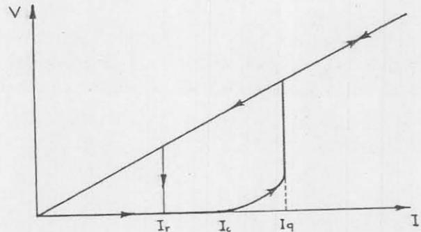
FIG. 3b - Current-voltage characteristics of a stabilized superconductor.
