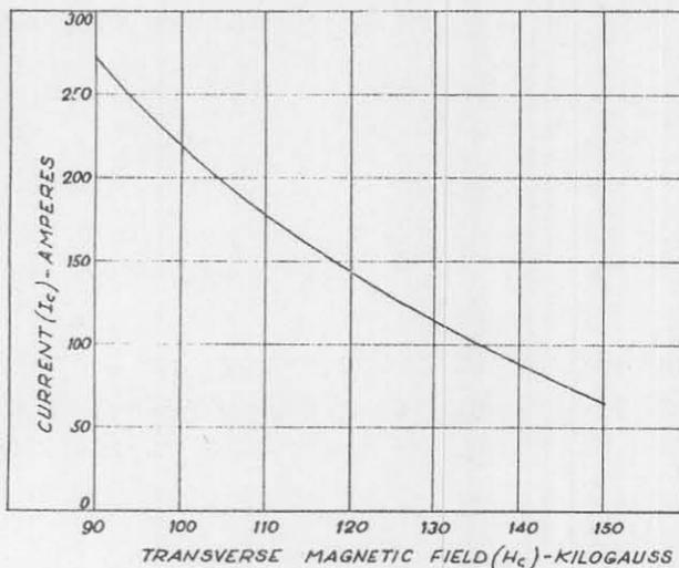
FIG. 1 - Critical current versus transverse magnetic field of a  $\text{Nb}_3\text{Sn}$  ribbon<sup>(1)</sup>,
