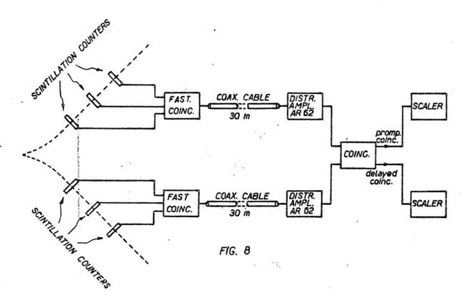
(4) The block diagram of electronics is shown in Fig. 8. Three-fold coincidences are obtained by means of the circuit shown in Fig. 9. The anodes of the tubes E180F are connected in parallel by means of inductances which form with stray capacitances an artificial transmission line of characteristic impedance  $Z_0$  and delay per section  $\tau_0$ .
