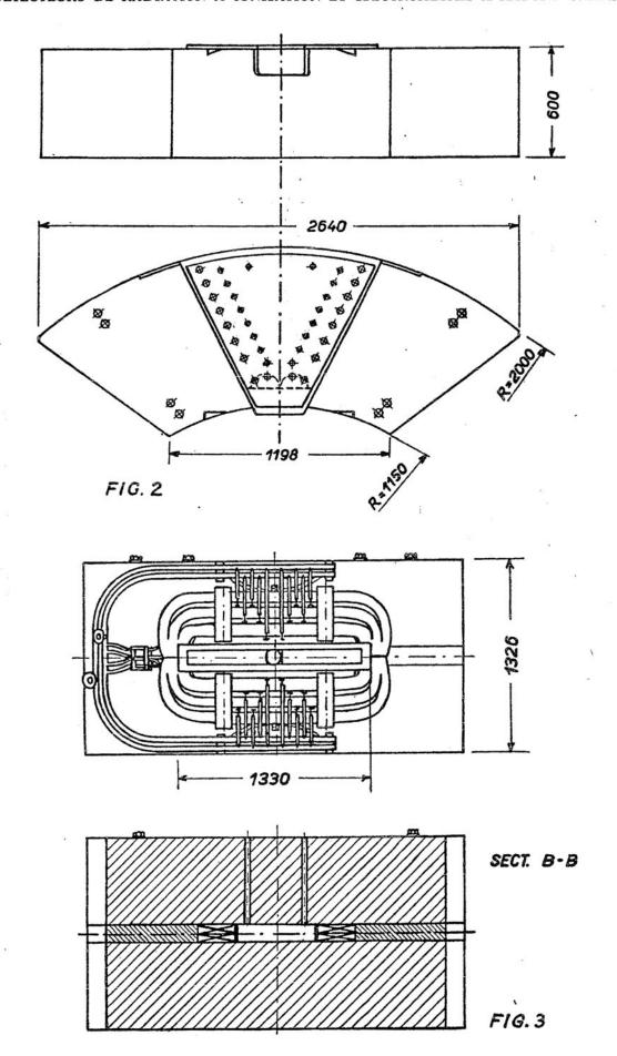
The magnet is shown in Figs. 1, 2 and 3; Fig. 1 shows the upper part, in which there are 36 holes for putting scintillation counters inside the magnet. The holes have been calculated to-obtain a multichannel pair spectrometer and for making electrodynamics experiments. The gap is 100 mm in height so that it should be possible to calibrate 60 mm beams. Around the gap a tank has been arranged in which a vacuum of the order of some tenth of mm Hg can be obtained.
