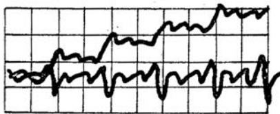
Fig. 8. Enlarged scale sweep 10 \mu\text{s}/\square , staircase (v.s. 1 \text{ volt}/\square = 9 \text{ gs}/\square ), pulses (v.s. 10 \text{ volt}/\square ).
