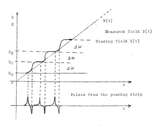
FIG. 2 - DIAGRAMS SHOWING THE PROCESS OF GENERATION OF THE STAIRCASE WAVEFORM.
