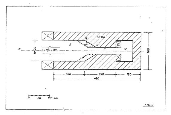
field in m-m' (see fig. 2) inside the limits of the fluxmeter (Pye Scalamp, precision 1%), and the general conclusion was that the final limit to the precision of the field in the region between A and B is mainly or only given by the precise control of the currents in coils I, II, III and in the correcting coils 3). The problem of realizing with the due precision the real a.c. excitation may be hard, and has not been completely examined as yet.
