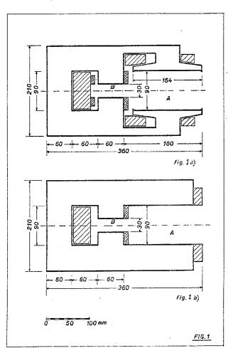
the schematic cross sections of two of the possible alternatives we considered in our note<sup>3</sup>). The possible distribution of the current conductors is indicated in the same note. With this distribution we should create a magnetic field with a constant and proper n-value in both the apertures A, B and in the region between the two gaps.
