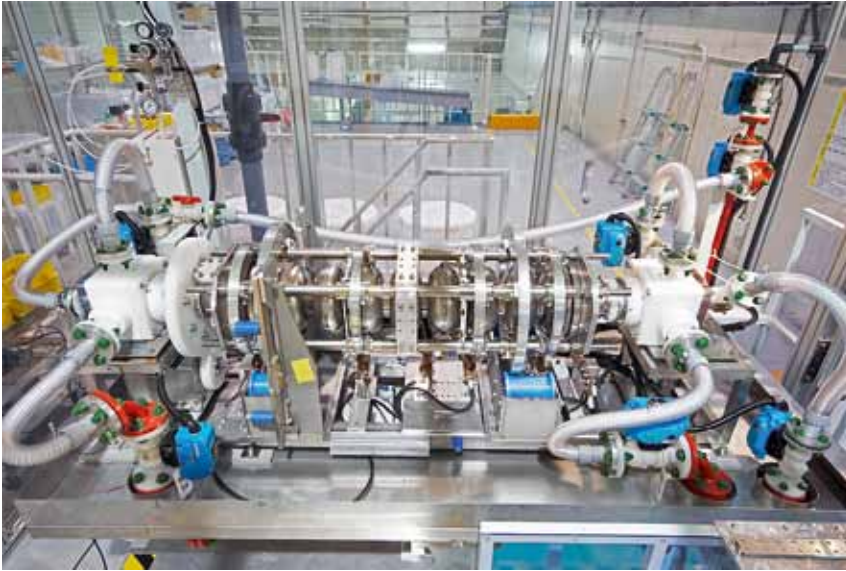
Figure 2.2 The EP facility established at KEK-STF.
