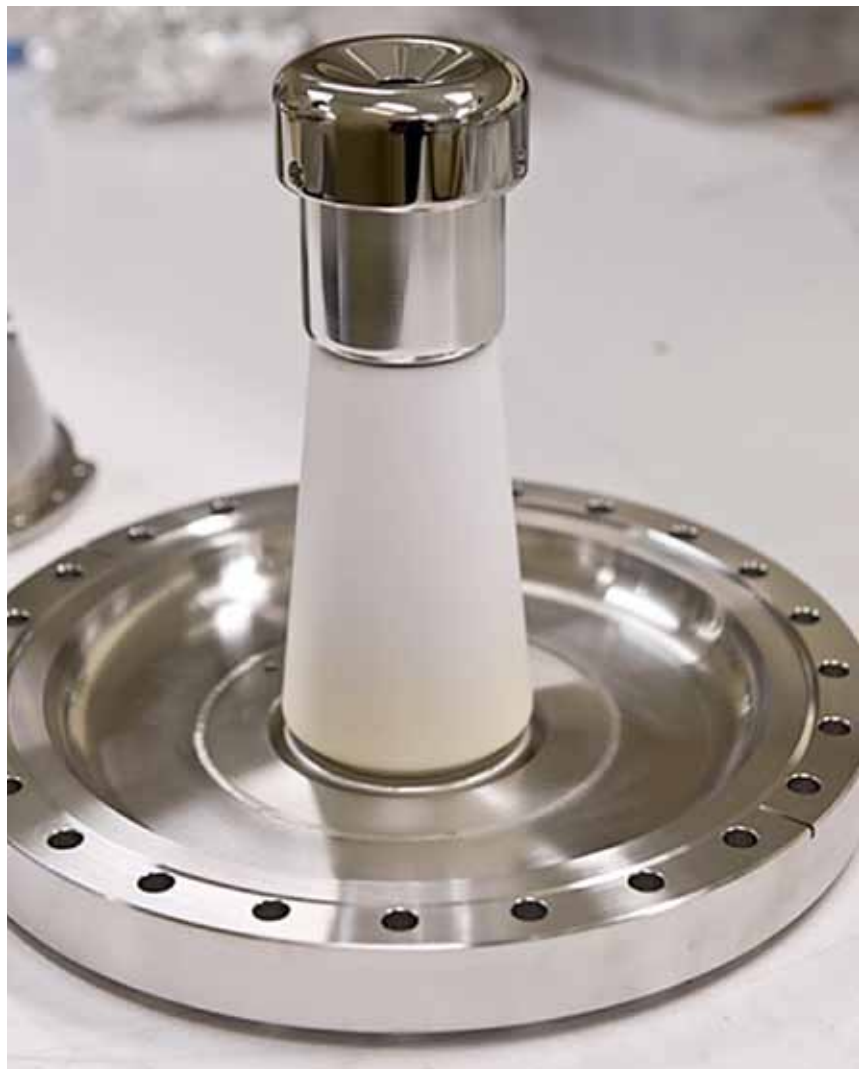
Figure 3.20 Niobium electrode of inverted gun design.
