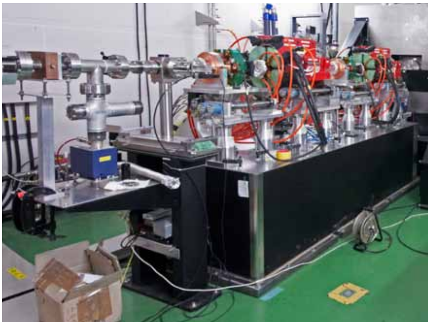
Figure 3.12 View of the final doublet installed on its rigid mechanical support system.
