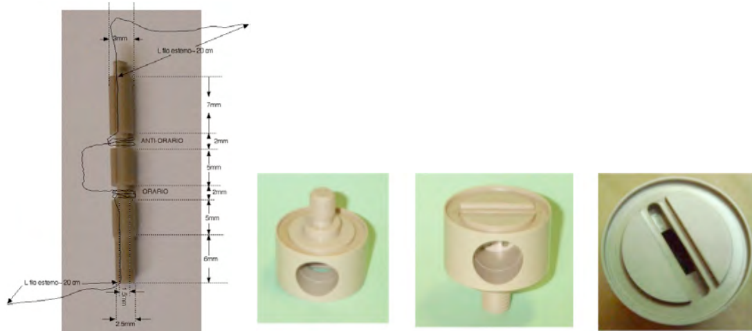
Figure 13: The first derivative PEEK gradiometer prototype (left); Different views of the PEEK DAC-holder (right).
