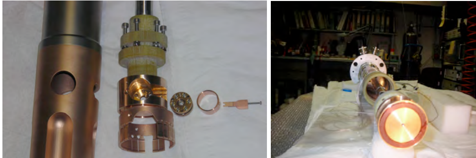
Figure 9: Photographs of the Cu-Be sample holder, the cold contact spring crown, the DAC and the slider (left) and the excitation coil (right)
