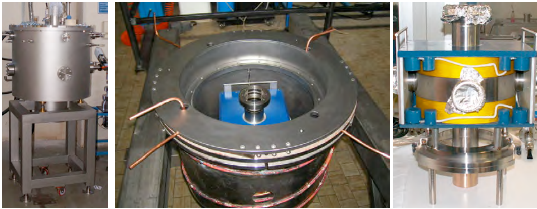
Figure 1: Photographs of cryostat (left), LN 2 shields, LHe vessel (center) and of the 8 T superconducting magnet (right) with the radial ports and the cold finger on the bottom.
