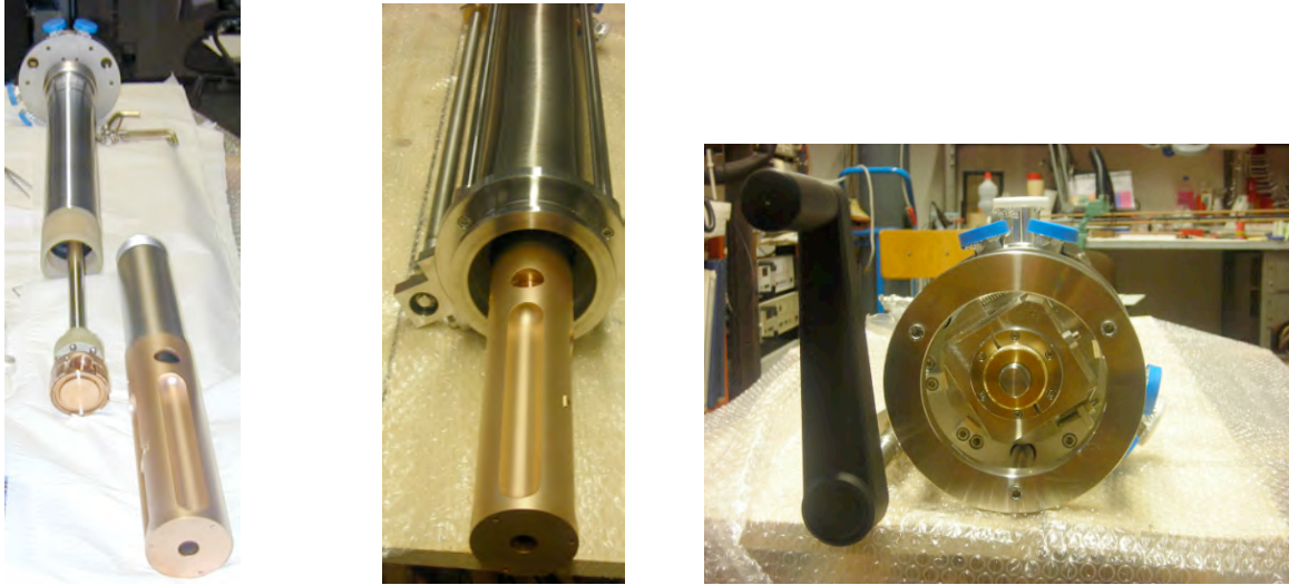
Figure 7: Photographs of the insert disassembled. The two main components (left), the long bellow for the vertical motion (central) and the X-Y- \Theta stage (right).
