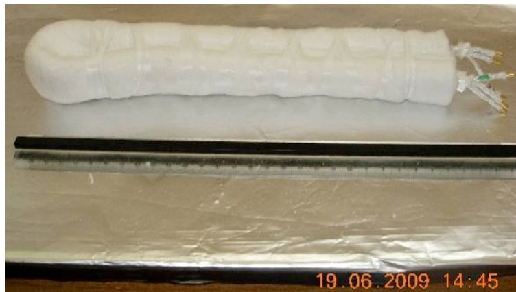
Fig 1: Wires braid inside the thermal insulation.
