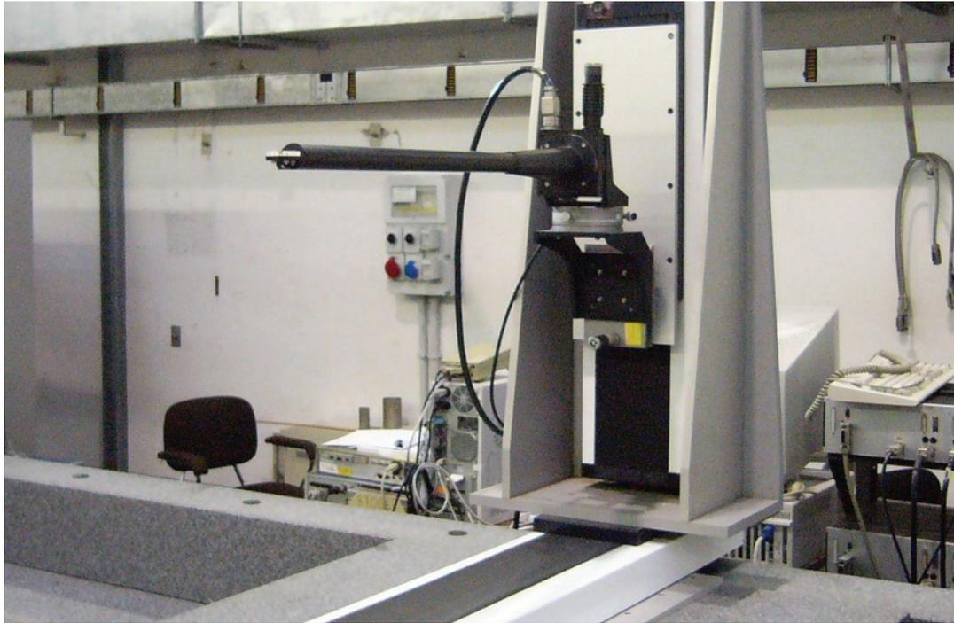
***Figure 11.7: Hall Probe Magnetic Measuring Machine***
