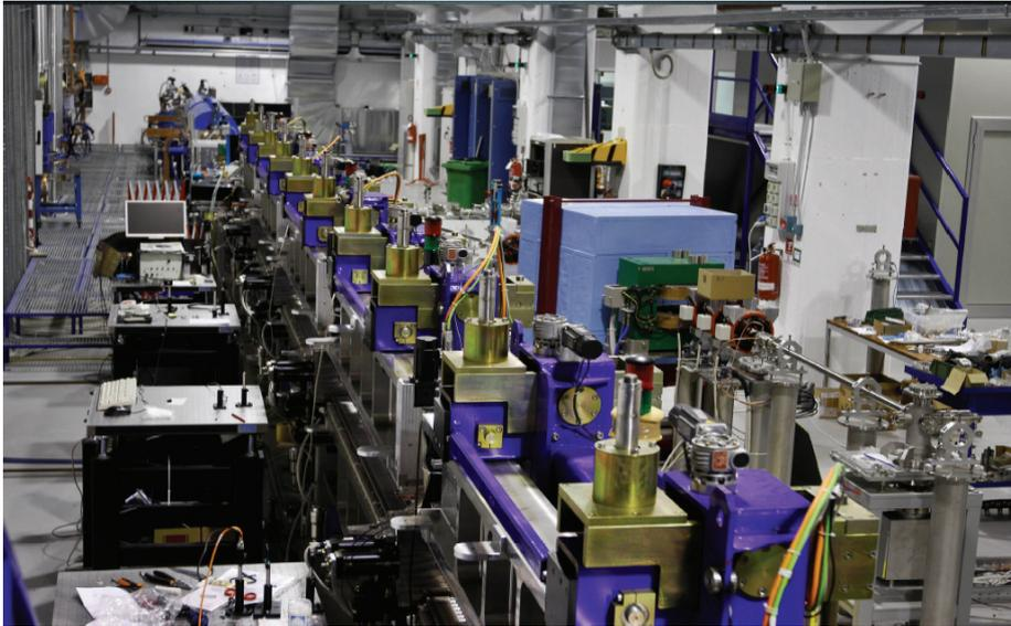
**Figure 3.29: Photo of the SPARC undulator sequence.**
