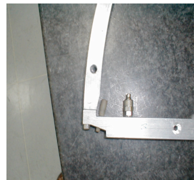
Fig. 5. The plastic joint (left) used to connect straw pieces, and the end-plug fixed to the mechanical frame (right).
