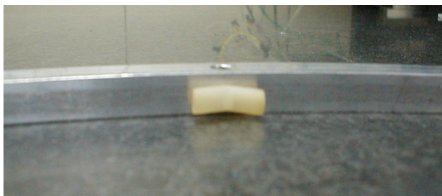
Fig. 5. The plastic joint (left) used to connect straw pieces, and the end-plug fixed to the mechanical frame (right).
