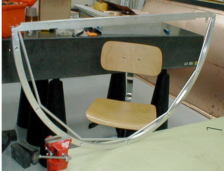
Fig. 4. First prototype of a segmented straw tube. The straw tube is mounted on a mechanical frame to allow a safe handling.
