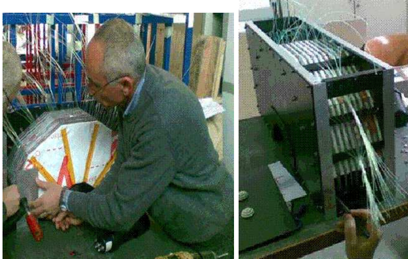
Fig. 5. Some pictures of a calorimeter module (five active sectors) assembly which took place in December 2007 and January 2008 at Frascati. The left picture shows the tiles wrapped in Tyvek™ sheets to improve the light collection efficiency; the WLS fibers, already bundled together and waiting for being connected to the PMT, are also apparent. In the right picture, the module has been put in its holding structure and is in the final building steps before being moved to the DAΦNE IP. The side view allows one to see the twelve scintillator planes such as the eleven lead layers.
