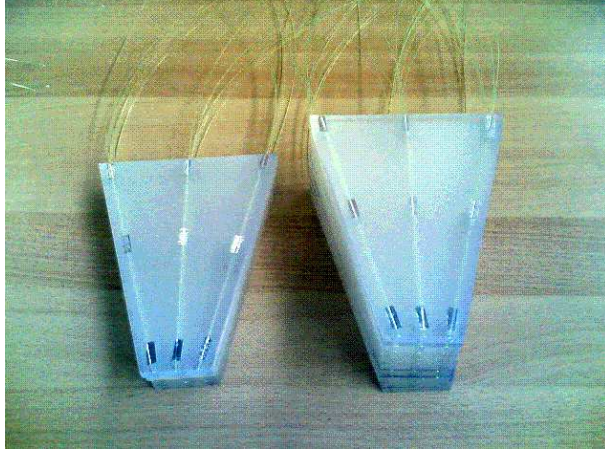
Fig. 4. Picture of calorimeter tiles with the WLS fibers already glued on their radial grooves.
