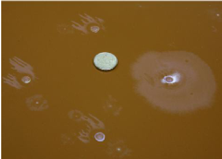
Figure 15: Large RPC chamber (2 m × 1 m) exposed at GIF with defects and oil drippings.
