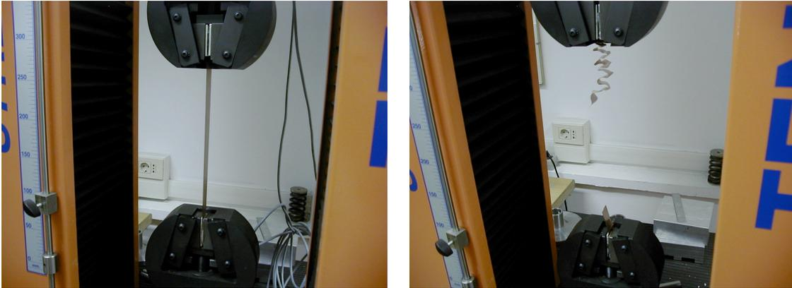
Figure 4: Tensile test on a specimen: during load application on the left and after break down, on the right.
