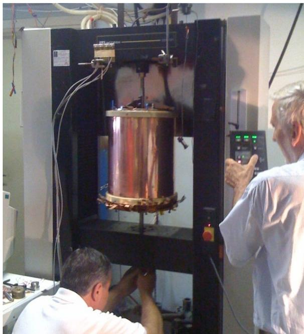
Figure 21: Full detector mounted on the ENEA tensile Machine.
