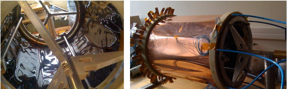
Figure 25: On the left: plastic deformation of the Catode cylinder most probably due to buckling instability, caused by external gas pressure; On the right: elastic buckling on the outer cylinder due to an external radial overpressure.
