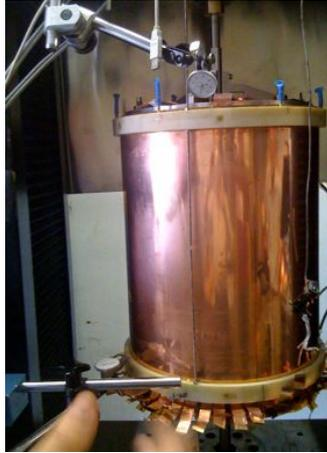
Figure 24: Experimental set-up for measurements with comparators
