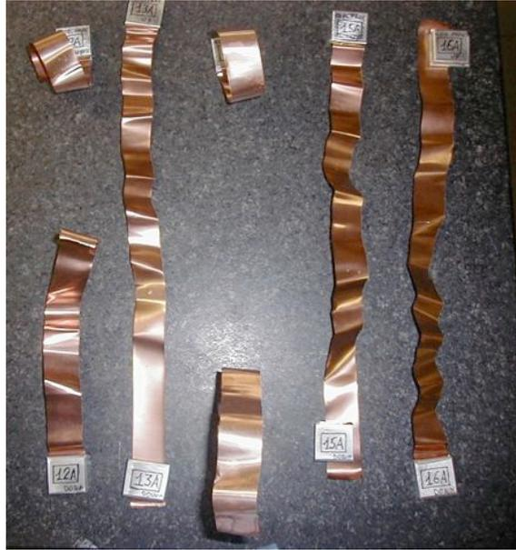
Figure 5: Anode specimens after tensile tests.
