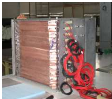
Figure 5: A picture of the GGM system ready to be shipped to CERN. The stack is enclosed into an aluminum box for further shielding.
