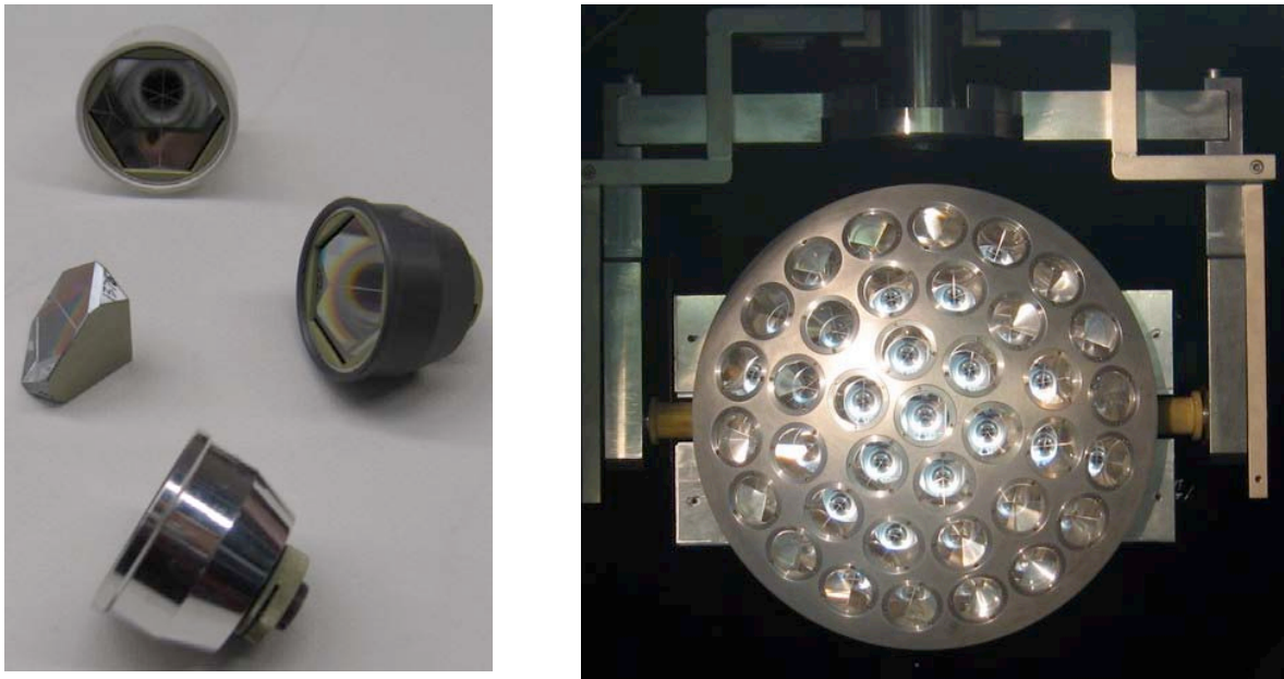
Figure 2 – Photos of three GLONASS (left) and LAGEOS Sector (right) prototypes.
