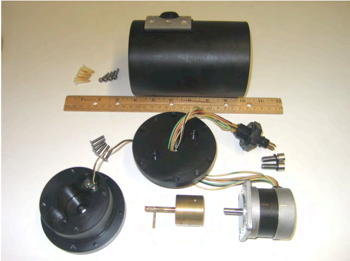
Fig. 7: The motor components, disassembled in the laboratory.
