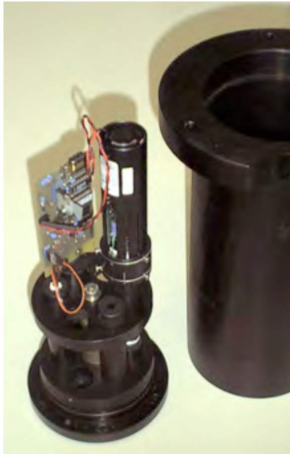
Fig. 10: NERONE DAQ BOARD and blue laser.
