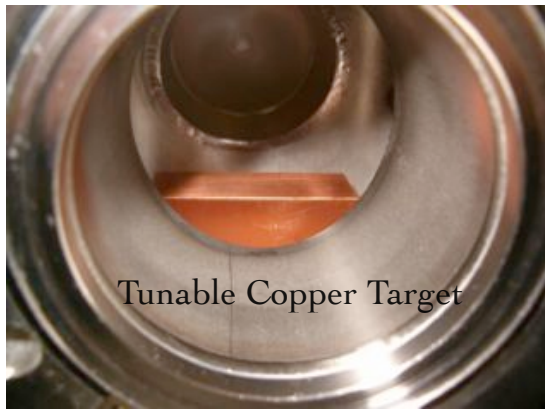
Figure 2: BTF copper target : in this picture it is completely kept away from the beam pipe.
