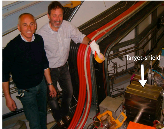
Figure 10: Target Shield installation (frontal view).
