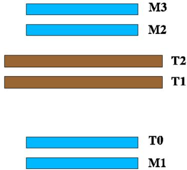
Figure 1: Sketch of the experimental set-up, with the trigger chambers (M1, M2, M3) and the three chambers under test (T0, T1, T2).
