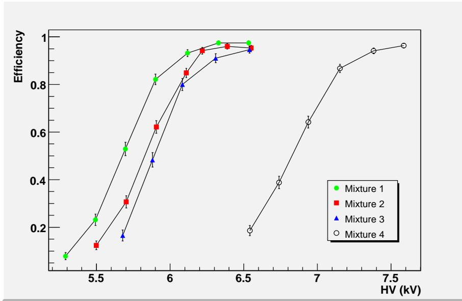
Figure 6: Efficiencies measured for mixtures with different isobutane concentrations.
