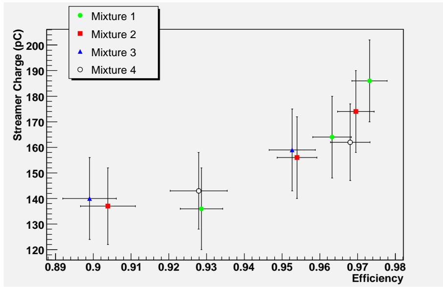
Figure 7: Streamer induced charge as a function of the efficiency for mixtures with different isobutane concentrations.
