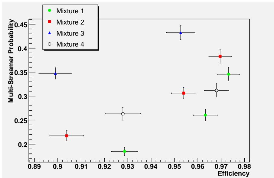
Figure 8: Multi-Streamer probability as a function of the efficiency for mixtures with different isobutane concentrations.
