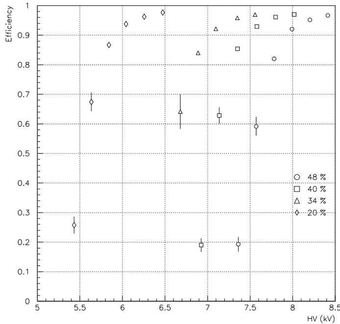
Figure 3: Efficiencies for different R134a concentrations in ternary mixtures with argon and isobutane (fixed at 4%).
