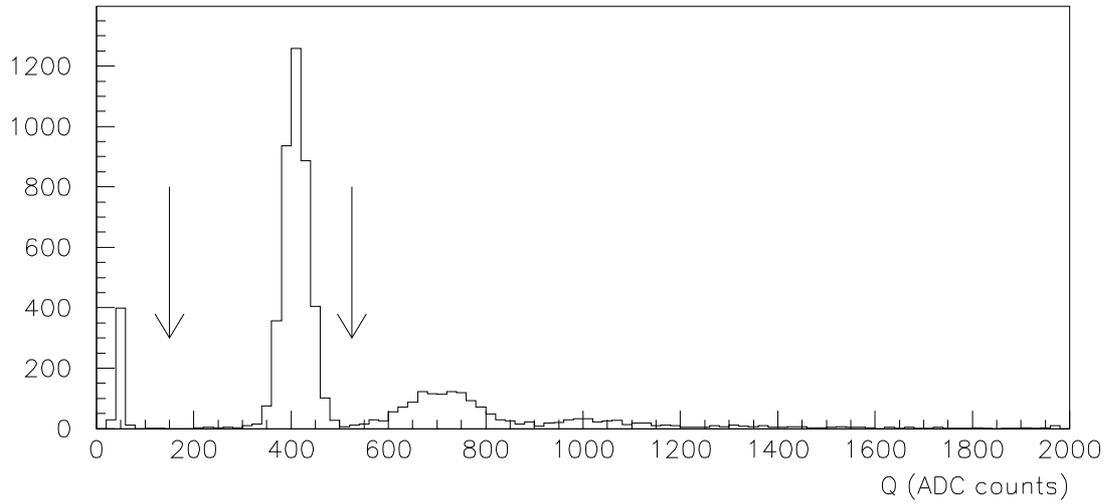
Figure 2: Induced charge for the gas mixture  $Ar/C_2H_2F_4/isoC_4H_{10} = 56/40/4$  at  $V=7.6$  kV. One ADC count is .83 pC. The cuts for selecting single streamers are also shown.
