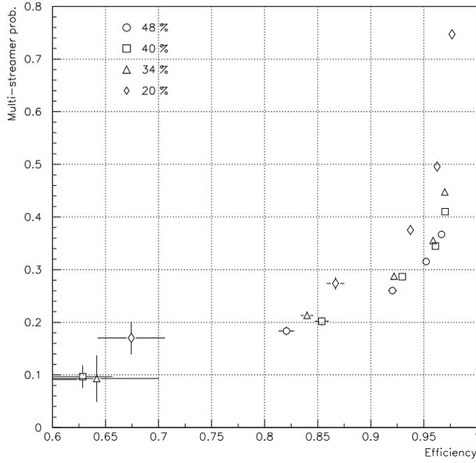
Figure 5: Multi-Streamer probability as a function of the efficiency for different R134a concentrations in ternary mixtures with argon and isobutane (fixed at 4%).
