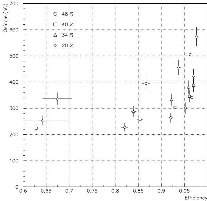
Figure 4: Streamer induced charge as a function of the efficiency for different R134a concentrations in ternary mixtures with argon and isobutane (fixed at 4%).
