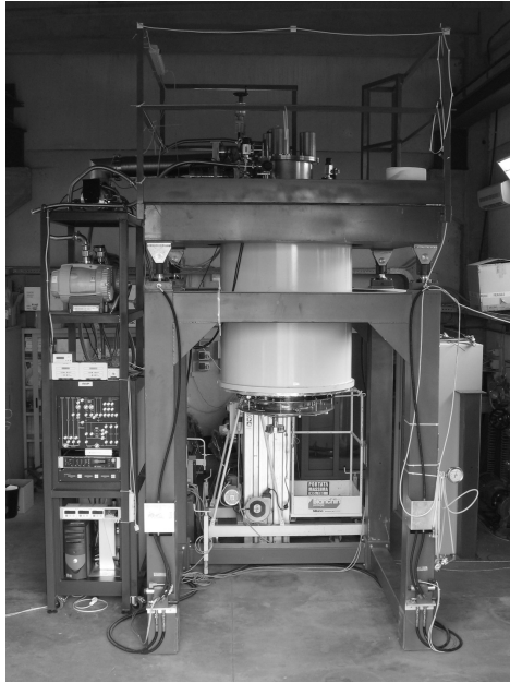
Figure 1: The RAP cryostat, with the experimental chamber opened. On the left the gas handling panel with the diagnostic electronics and the PC are shown. Above the panel stands the pumping system.
