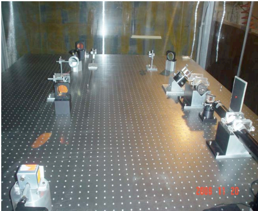
Figure 20. The optical table to evaluate the optical performance of the CCRs.
