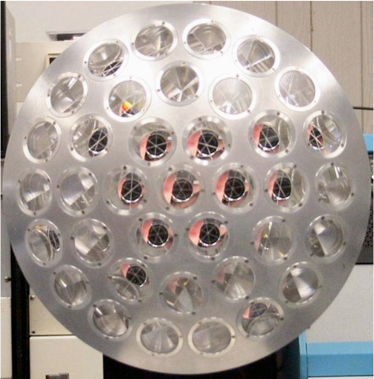
Figure 2.13 – LAGEOS cap at LNF –
