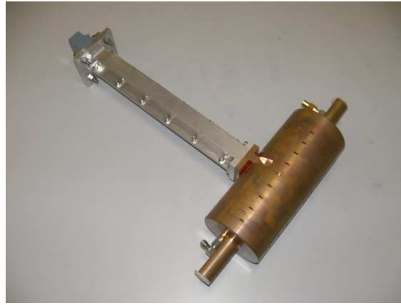
Figure 1: Brazed periodic cavity prototype.
