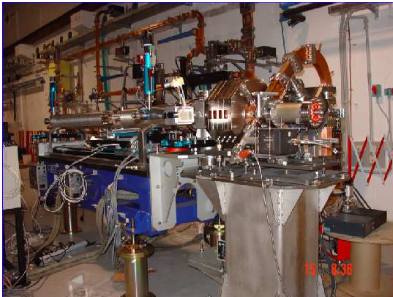
Figure 2: Picture of the SPARC photoinjector showing the RF gun with solenoid and emittance meter installed.
