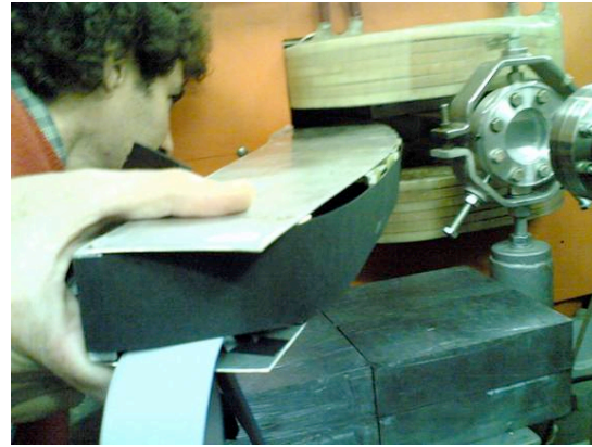
Figure 6: Insertion of the new set-up inside the bending dipole
