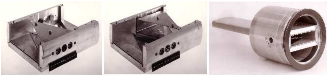
Figure 1: SPS beam position monitor slant-cut diagonally.
