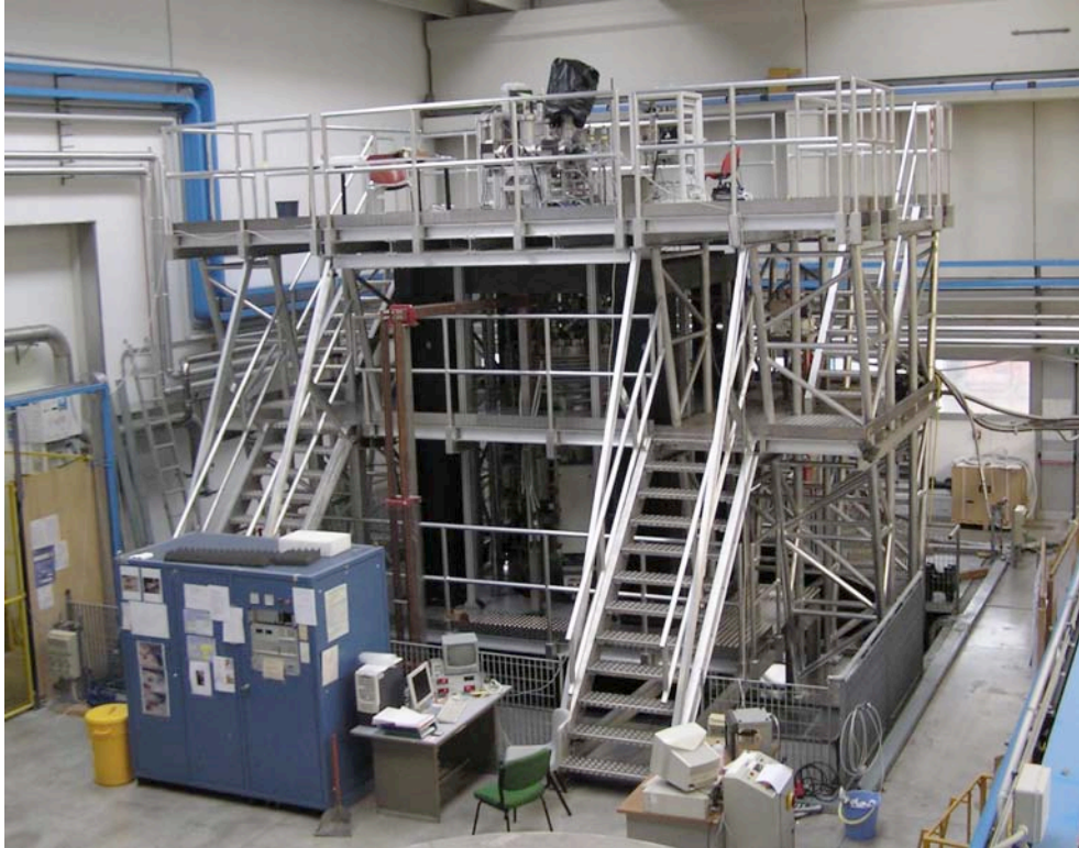
Figure 1: View of the PVLAS optics tower showing the new aluminum access structure.
