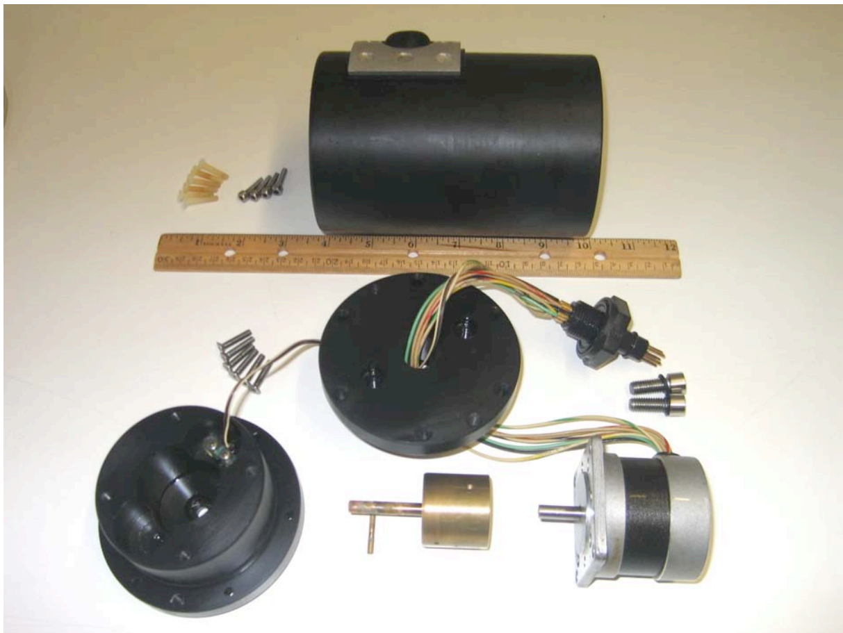
Fig. 4: The motor components, disassembled in the laboratory.
