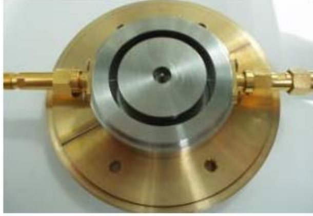
Figure 24: A prototype of the re-entrant cavity transducer ready for testing. Note the clamps that keep the cavity tight onto the reference plane and the rf connectors that deliver the power and extract the signal. The cavity can be tested both in two-port configuration (transmission) and in one-port configuration (reflection).
