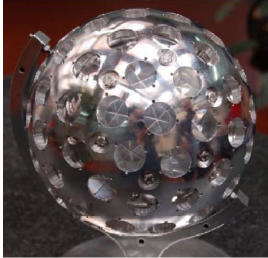
Fig. 10. The 1:2 scale prototype of the new shell-over-the-core LARES design built at LNF.
