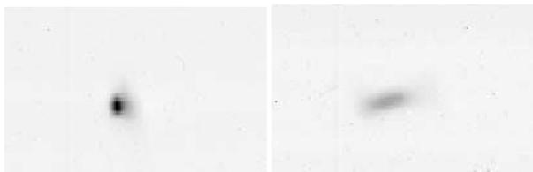
Figure 9: Unprocessed bunch images. Left: RFD switched off. Right: RFD on, at zero-crossing phase.
