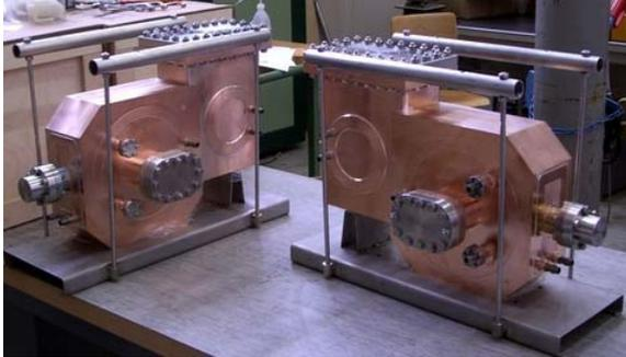
Figure 3: Picture of the two RF cavities of the deflector.
