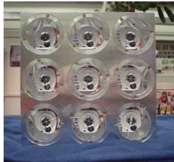
Figure 2: The LAGEOS 3x3 retro-reflector (CCR) matrix prototype.
