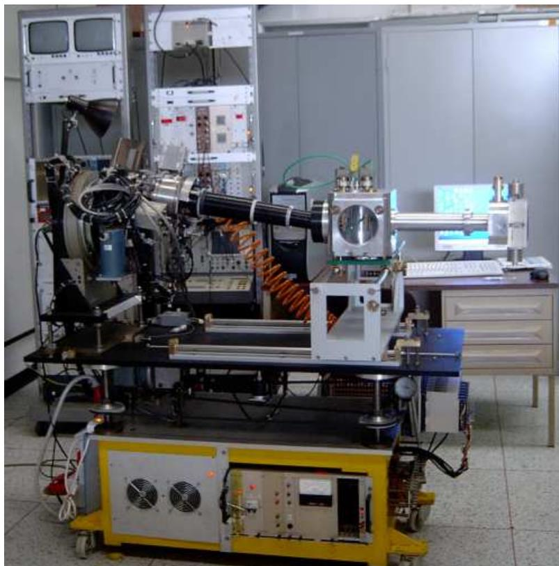
Figure 1: *The Small Angle X-ray Camera.*
