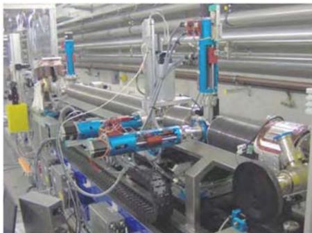
Figure 6: *SPARC e-meter during installation at the Photo Injector Test Facility PITZ.*
