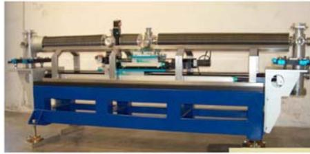
Figure 4: *Emittance-meter device with long bellows.*
