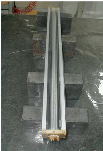
Figure 2: Photograph of the straw tube prototype constructed at the LNF.
