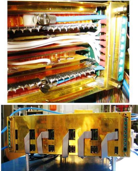
Figure 7: Top: Close view of the HV plug integrated on the faraday cage. Bottom: Picture of the final faraday cage of the detector station.
