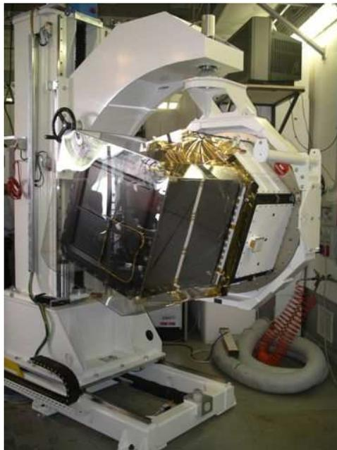
Figure 2: The AGILE instrument and upper part of the satellite on the gamma ray photon beam at the BTF, November 3, 2005
