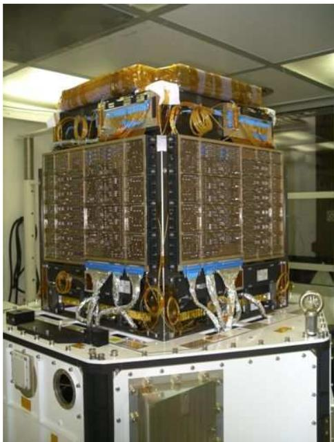
Figure 1: The AGILE detector integrated on the upper part of spacecraft
