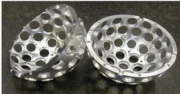
Figure 5: The outer half-shells of the new satellite design for the LARES space mission.
