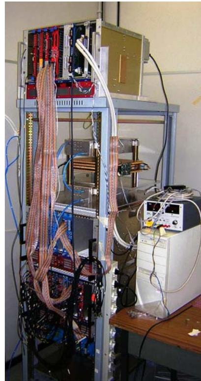
Figure 8: Picture of the cosmic ray setup used to measure the final station performances.
