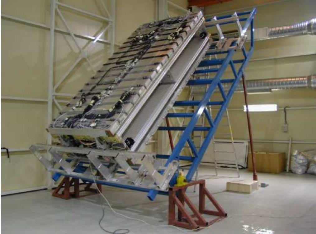
Figure 3: *Sag adjustment performed on a MDT station.*
