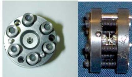
Figure 3: Photos of the diamond anvil cell (DAC). Top (left) and side (right) views.
