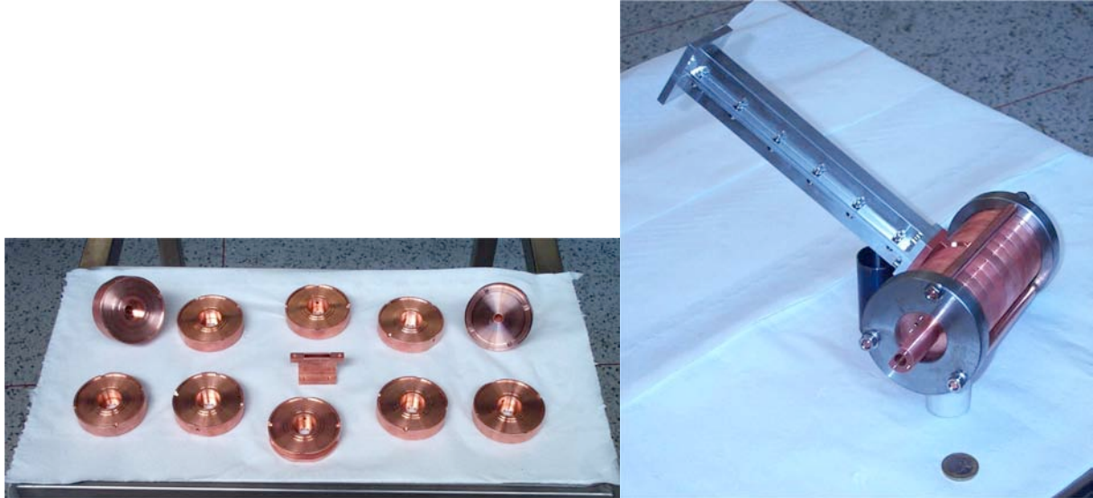
FIG. 11: copper prototype of the X band structure.
