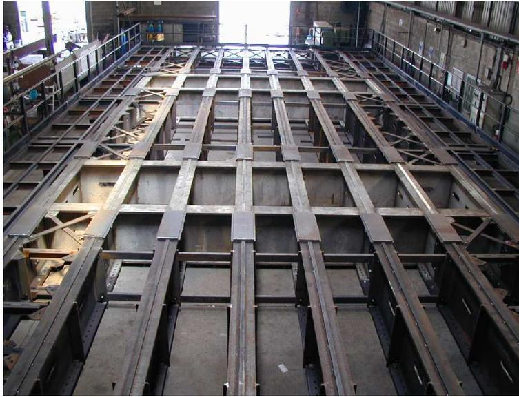
Figure 2: The support structure in the factory before transportation at LNGS.
