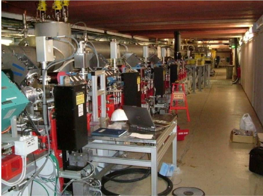
Figure 1: *The injector FODO structure with the 4 OTR screens for the emittance measurement.*
