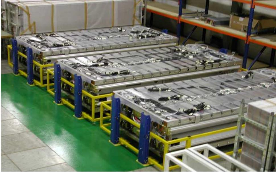
Figure 4: *MDT-RPC integrated station in the storage frame in the hall BB5 at CERN.*
