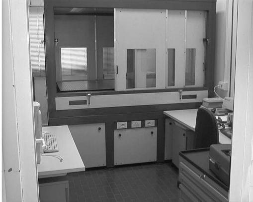
Figure 1: Cabinet with a “research grade” optical table to be used for characterization of different kind of X-ray optics.
