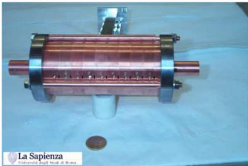
Figure 4: *SPARC* prototype of the nine cells IV Harmonic cavity.
