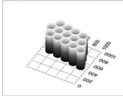
Figure 8: 3-D reconstruction in Tomo reference of the 14-straw module.
