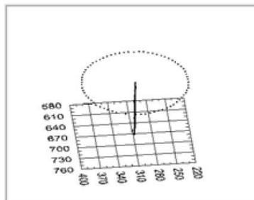
Figure 6: Axis and Edges of Section #130 of the straw tube #4 in Tomo reference. The Straw axis is at 9 degree respect to the tomograph vertical axis (the figure axis is not in scale respect the horizontal ones)
