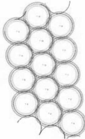
Figure 5: Edges of 14 straw tubes of the section #10 of the module. Each Edge is chosen as the first met in the arrow direction, from the inside to the outside of the Region of Interest, pointing out to the internal surface of the straw tube. Circles fitting the Edges, their centers and order number are also shown
