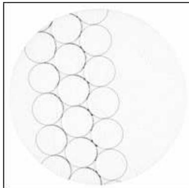
Figure 1: Example of raw tomography image of straw tubes module (1024x1024 pixel,  $27\mu\text{m}/\text{pixel}$ )
