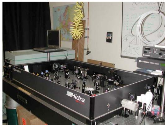
Figure 3: HIDRA-50 amplifier for the SPARC laser.
