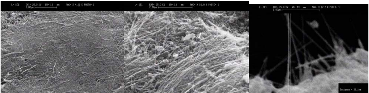
Fig. 1 SEM images of a cathodic deposit obtained at LNF by arc-discharge.
