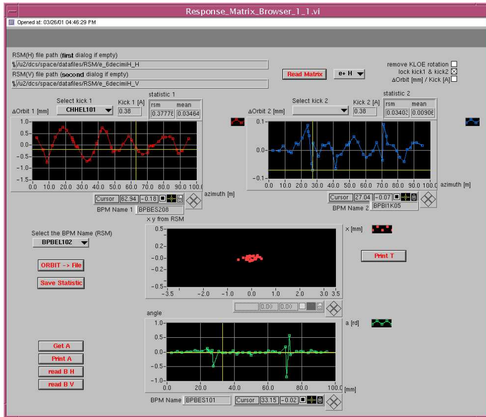
Figure 7.2: The LabView program window of the DAΦNE control system that measures the closed orbit response matrix.
