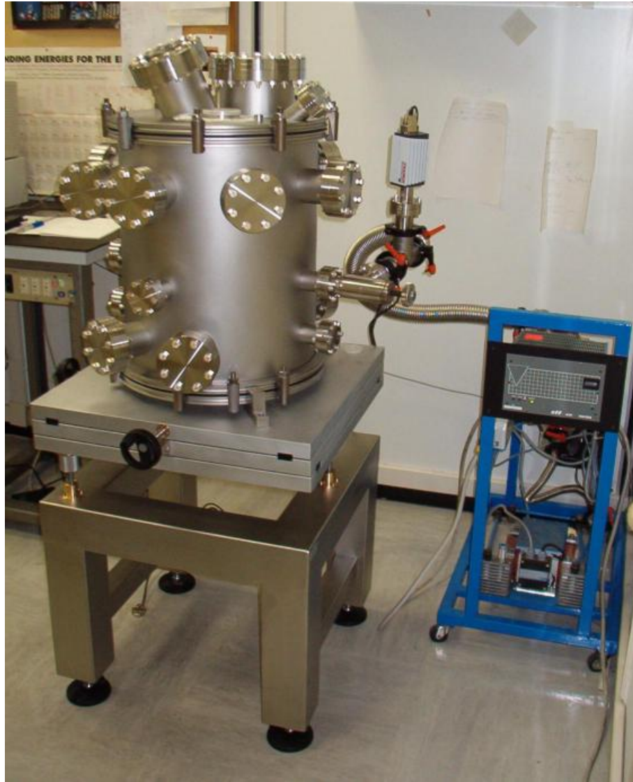
Figure 5: The experimental chamber and its support during the preliminary vacuum tests at Frascati.
