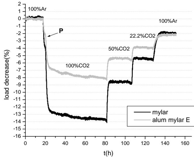
**FIG. 12:** Mylar and aluminised mylar E load decrease (%) for four different CO<sub>2</sub> percentages of the gas mixture. In P mixture is set at 22.2%CO<sub>2</sub>, but after 2 hours Ar bottle finishes and mixture becomes 100% CO<sub>2</sub> before reaching stability.
