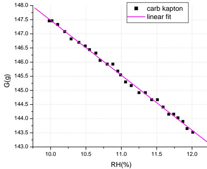
**FIG. 10:** Scatter plot example of tension vs RH for carbonated kapton in 100%CO<sub>2</sub> (20 l/h).
