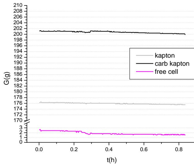
**FIG. 5:** Kapton, carbonated kapton and free cell trends when flow rate is changed from 40 l/h to 80 l/h for a gas mixture of 22.2%CO<sub>2</sub>+ 77.7%Ar.
