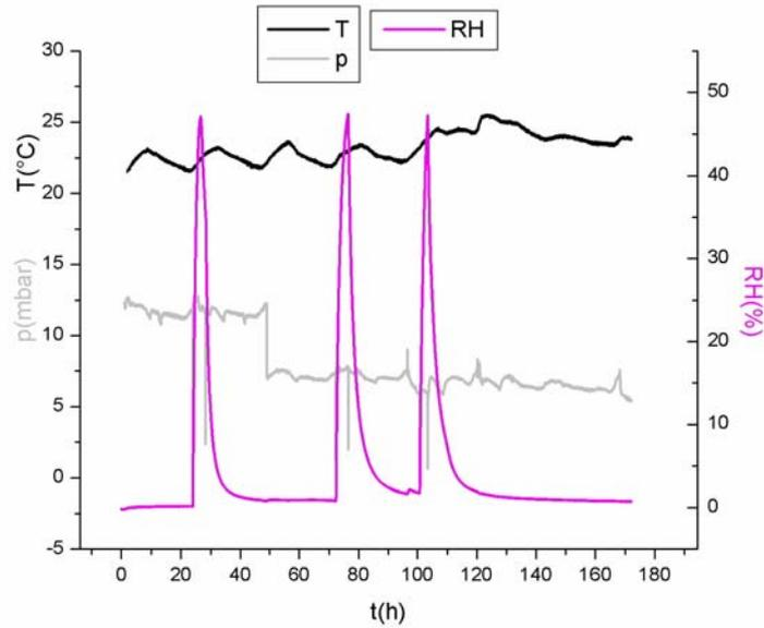
**FIG. 6:** T, p, RH trends for three humidity tests: the first peak is in 22.2% CO<sub>2</sub> (34.3 l/h), the second in 100% Ar (20 l/h), the last in 100% CO<sub>2</sub> (20 l/h). The down-peaks of pressure represent the connection and disconnection to the small water bottle.
