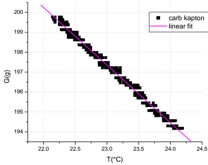
**FIG. 2:** Scatter plot example of tension vs temperature for carbonated kapton in CO<sub>2</sub>.
