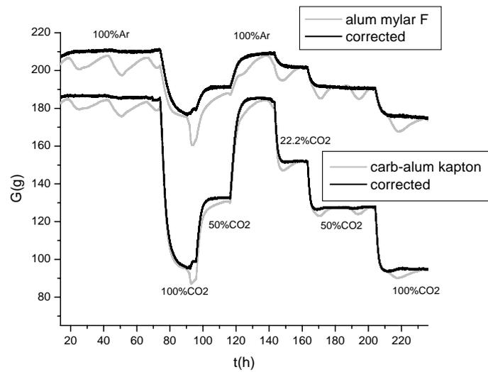
**FIG. 3:** T correction for aluminised mylar F and carbonated aluminised kapton in different Ar-CO<sub>2</sub> mixture.
