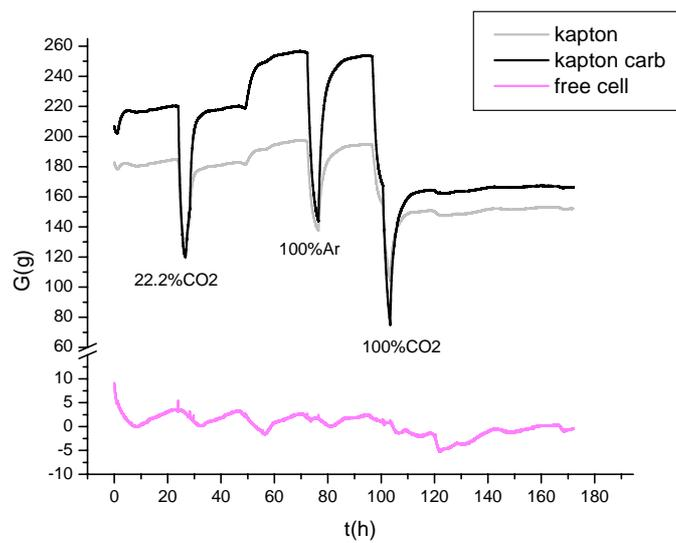
**FIG. 7:** Kapton, kapton carbonate and free cell trends during humidity test.
