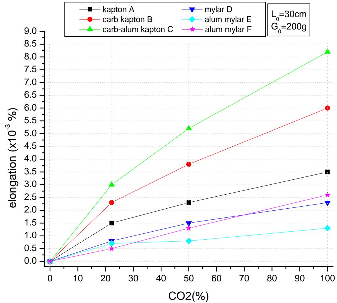
**FIG. 14:** Strips elongation (%) at four different gas mixtures of CO<sub>2</sub> and Ar: 100%Ar, 22.2%CO<sub>2</sub>, 50%CO<sub>2</sub> and 100%CO<sub>2</sub>.
