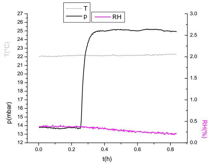
**FIG. 4:** T, p, RH trends when flow rate is changed from 40 l/h to 80 l/h for a gas mixture of 22.2% CO<sub>2</sub>+ 77.7% Ar.
