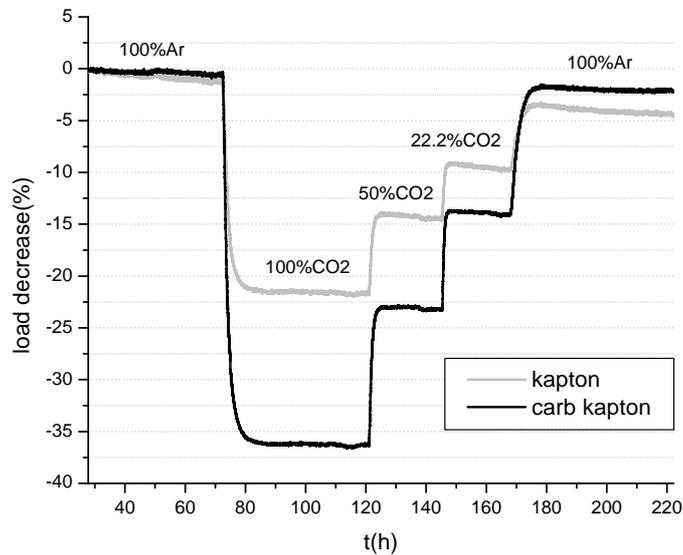
**FIG. 11:** Kapton and carbonated kapton load decrease (%) for four different CO<sub>2</sub> percentages of the gas mixture.
