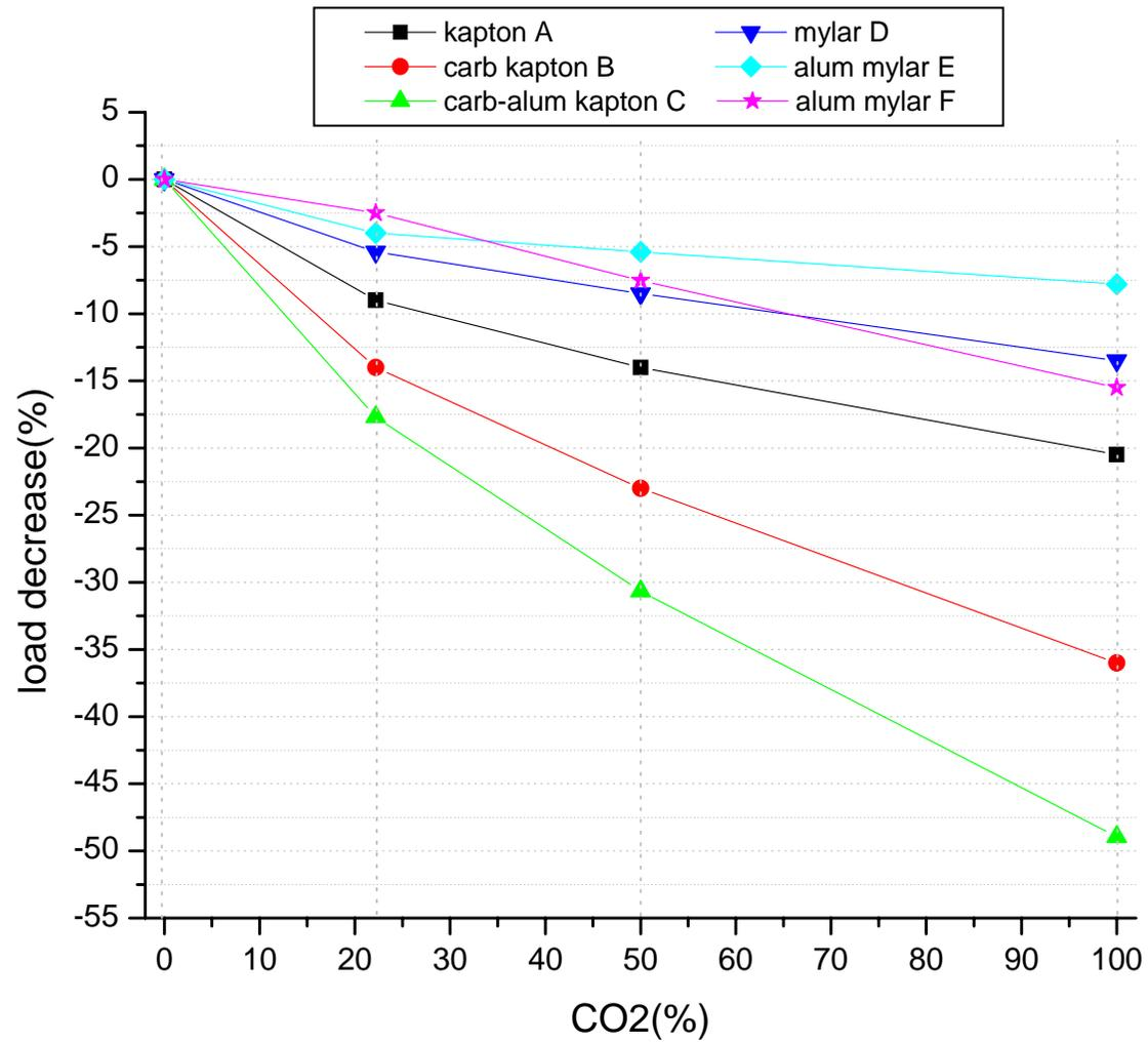
**FIG. 13:** Strips load decrease (%) at four different gas mixtures of CO<sub>2</sub> and Ar: 100%Ar, 22.2%CO<sub>2</sub>, 50%CO<sub>2</sub> and 100%CO<sub>2</sub>.
