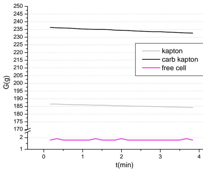
**FIG. 9:** Kapton, carbonated kapton and free cell trends during RH humidity change from 10% to 12% in 100% Ar (20 l/h).
