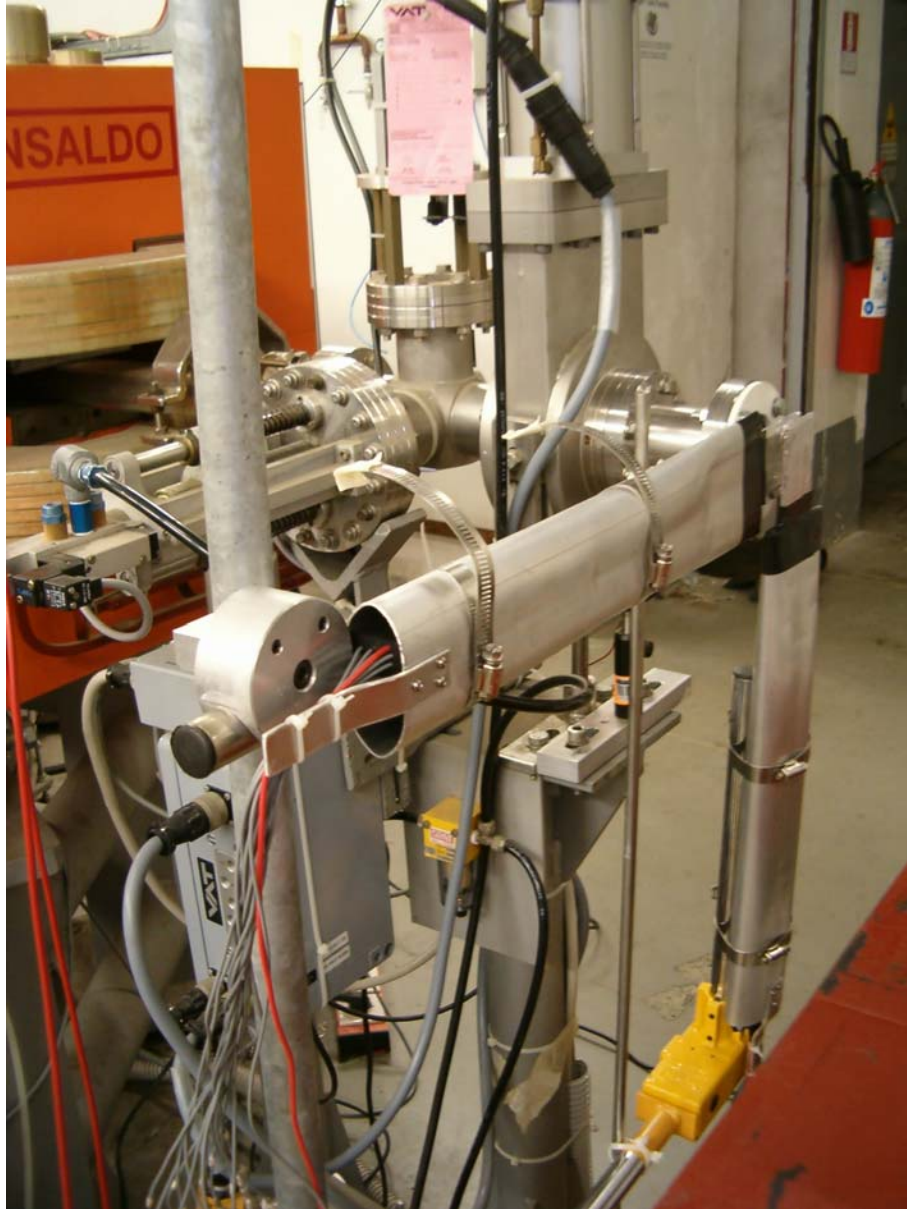
Figure 7: The two views of the fiber detector assembled together with the fibers running horizontally ( y view) and vertically ( x view) in the plane perpendicular to the beam direction.
