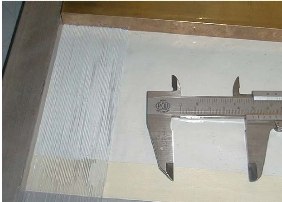
Figure 2: Gluing one layer of 48 scintillating fibers.
