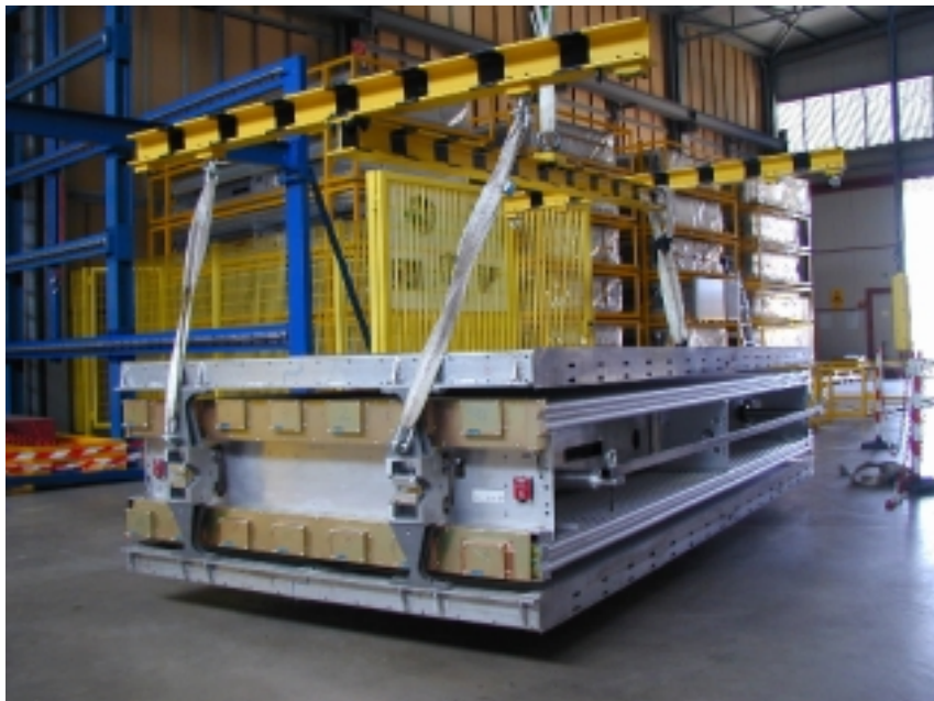
Figure 12: The MDT RPC integration realized by the common supports designed at the LNF.
