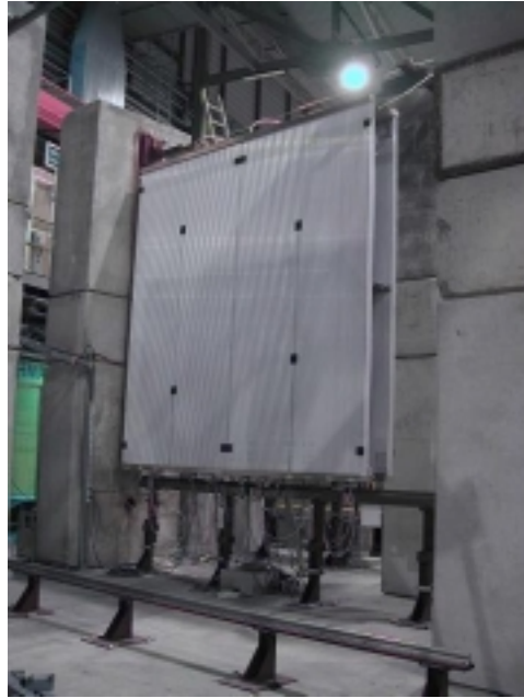
Figure 7: The set-up of the H8 test beam at CERN showing the two fully equipped BML chambers produced at the LNF.
