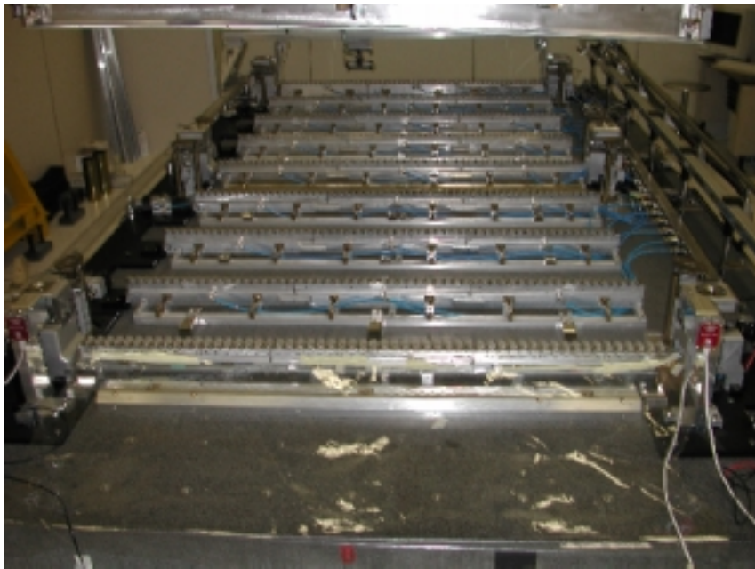
Figure 1: The high precision jig for the positioning of the tubes.
