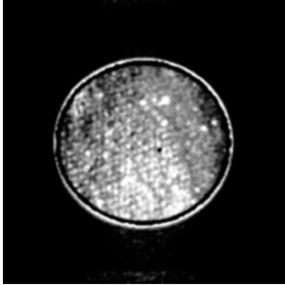
Figure 2: The picture shows in detail the GEM pinhole structure with diameter \sim 50\mu\text{m} , resolved by the CCD matrix, whose pixel size is \sim 20\mu\text{m} .
