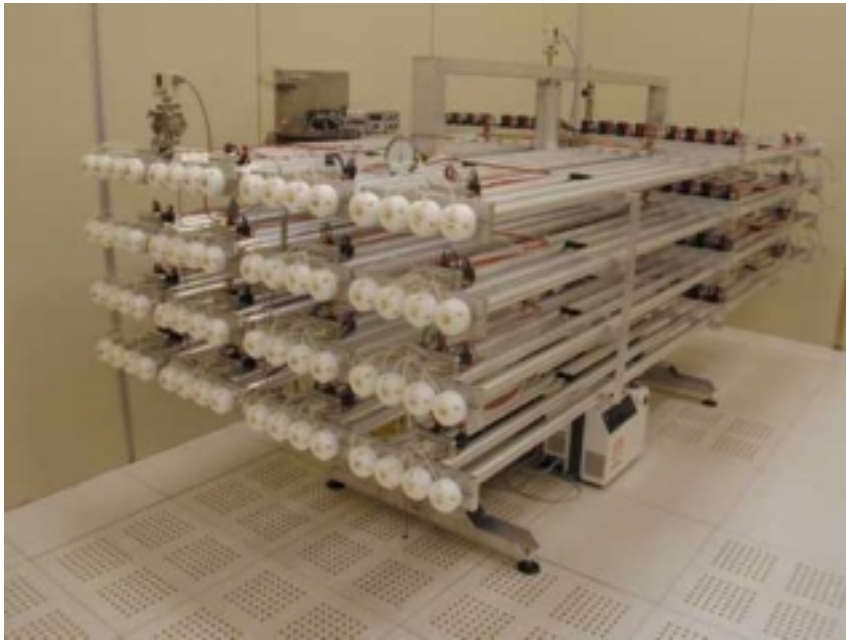
Figure 3: The gas leak test station based on a helium spectrometer.
