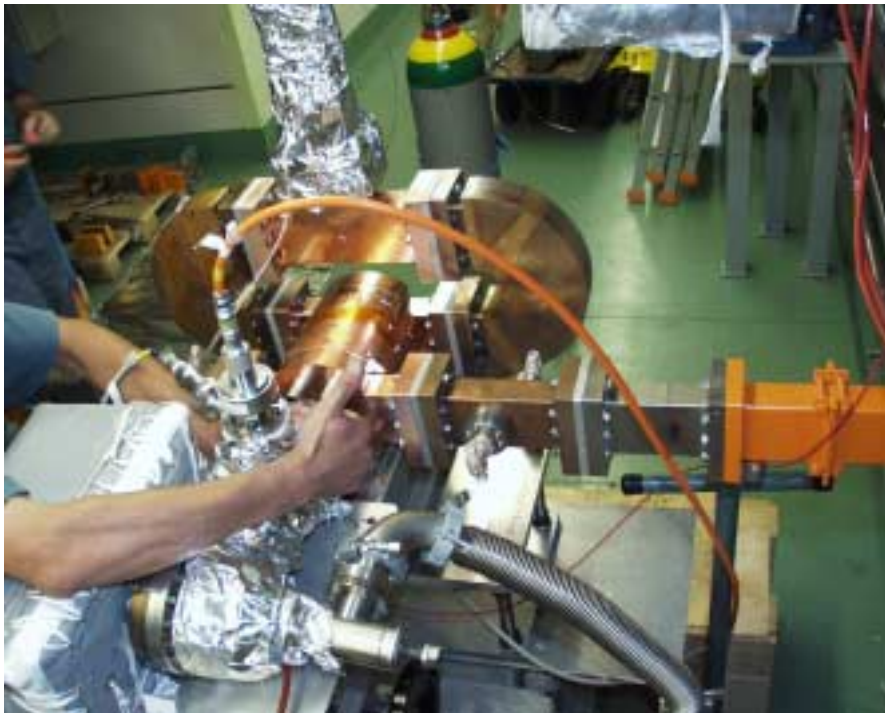
Figure 9.8: Short SICA prototype being prepared for high power tests in the CTF3 tunnel
