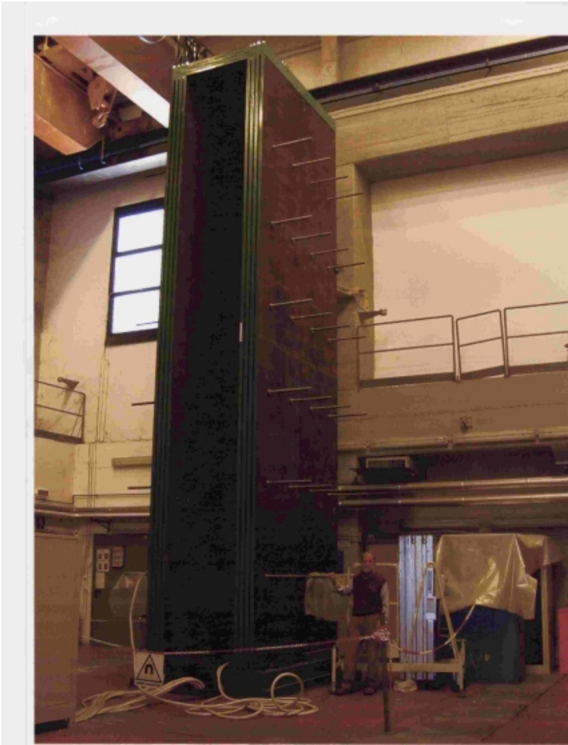
Figure 1: The OPERA dipolar magnet prototype.
