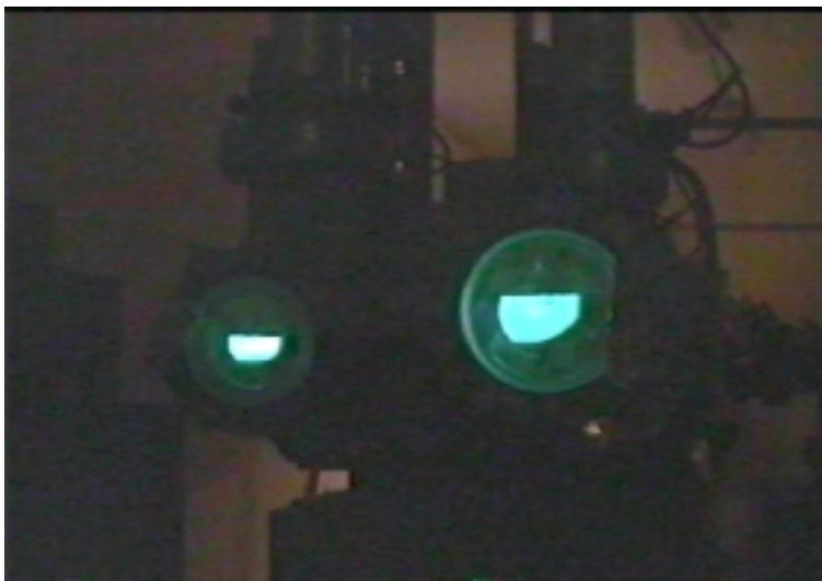
Figure 5: The two visible spots shown in the photo are the light emitted by the phosphorus excited by the two SR X-ray beams striking the two viewports
