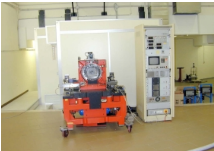
Figure 2: The Karl SUSS x-ray stepper.
