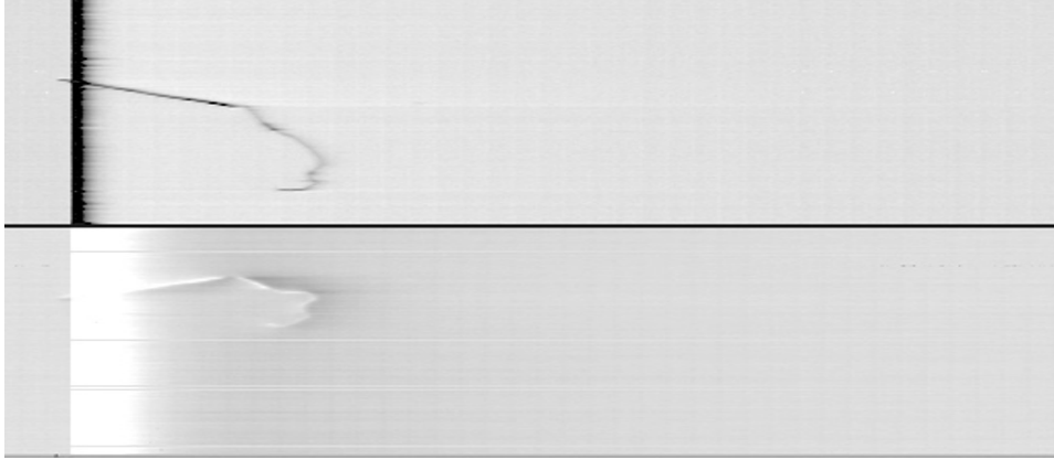
Figure 1: Picture of a stopping \mu^+ event, showing the decay into a positron. This type of event gives a characteristic double light pulse, one associated with the incoming muon, the other, on average 2.2\mu\text{s} later, associated with the decay into e^+ . Both the charge collection and the charge induction views are showed here. Note the visible time delay between the muon stopping point and the electron starting point.
