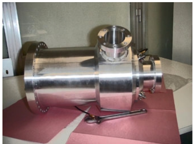
Figure 2: Picture of the harmonic cavity prototype
