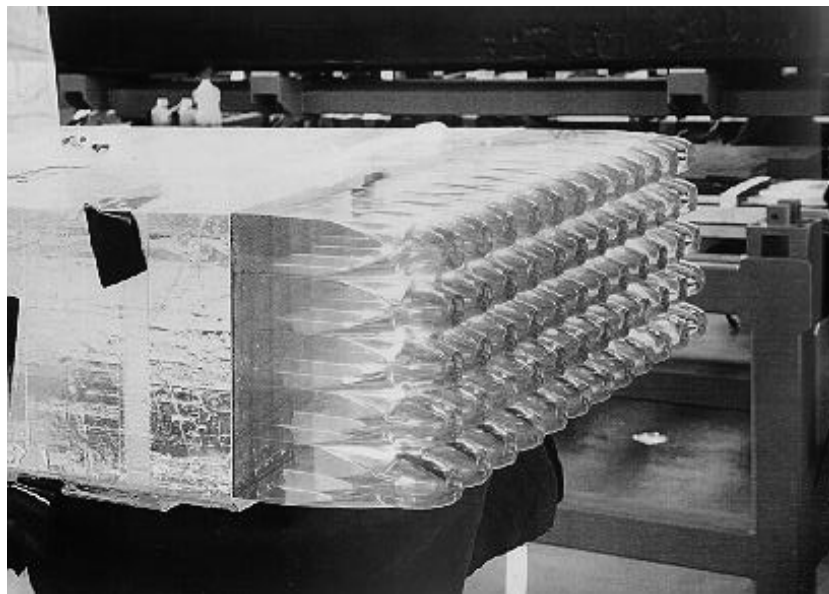
Figure 3. Light guides at one end of a barrel module before photo-tube installation.
