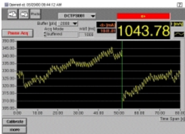
Figure 3: DCCT current record in the positron ring.
