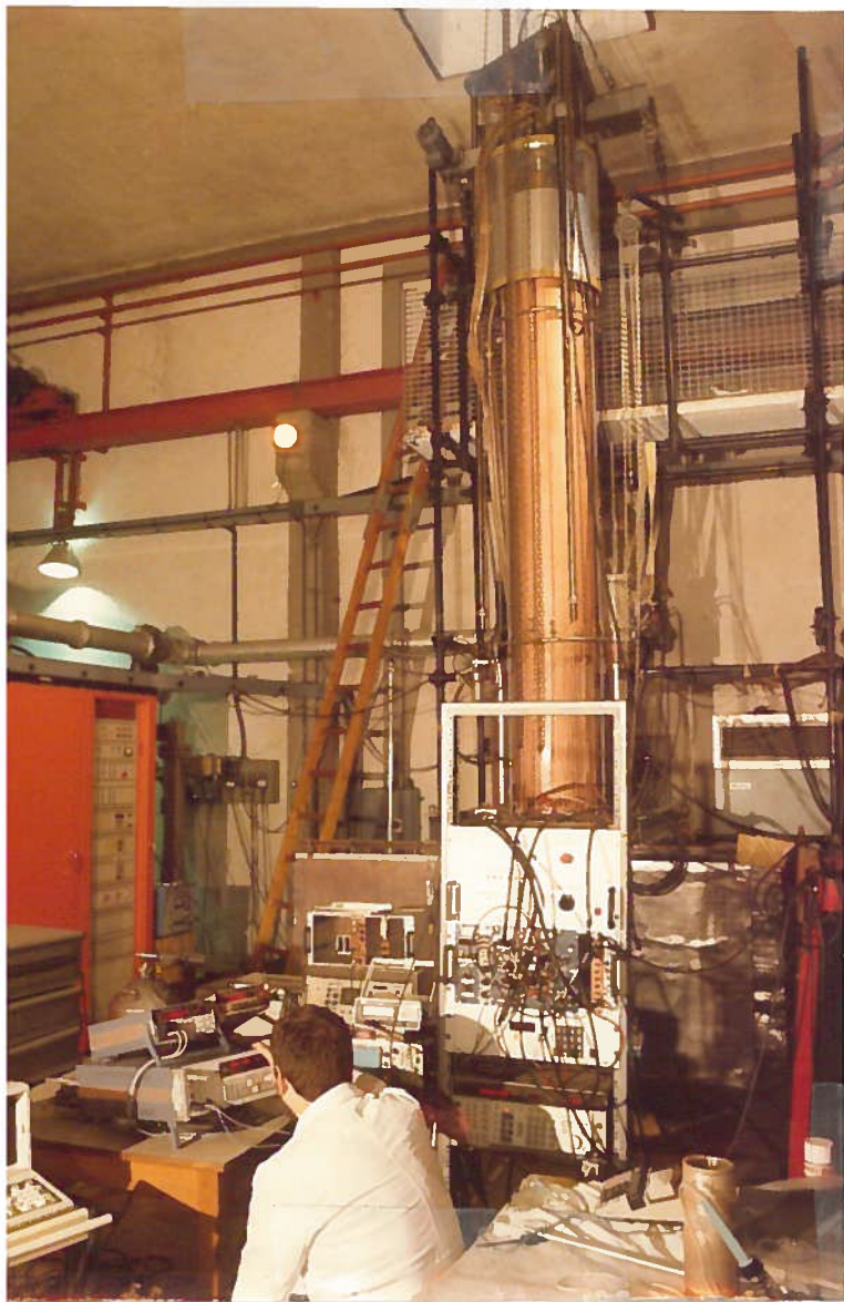
FIG. 13 - The first RF cavity (upper half) under power tests, connected to the control electronics.
