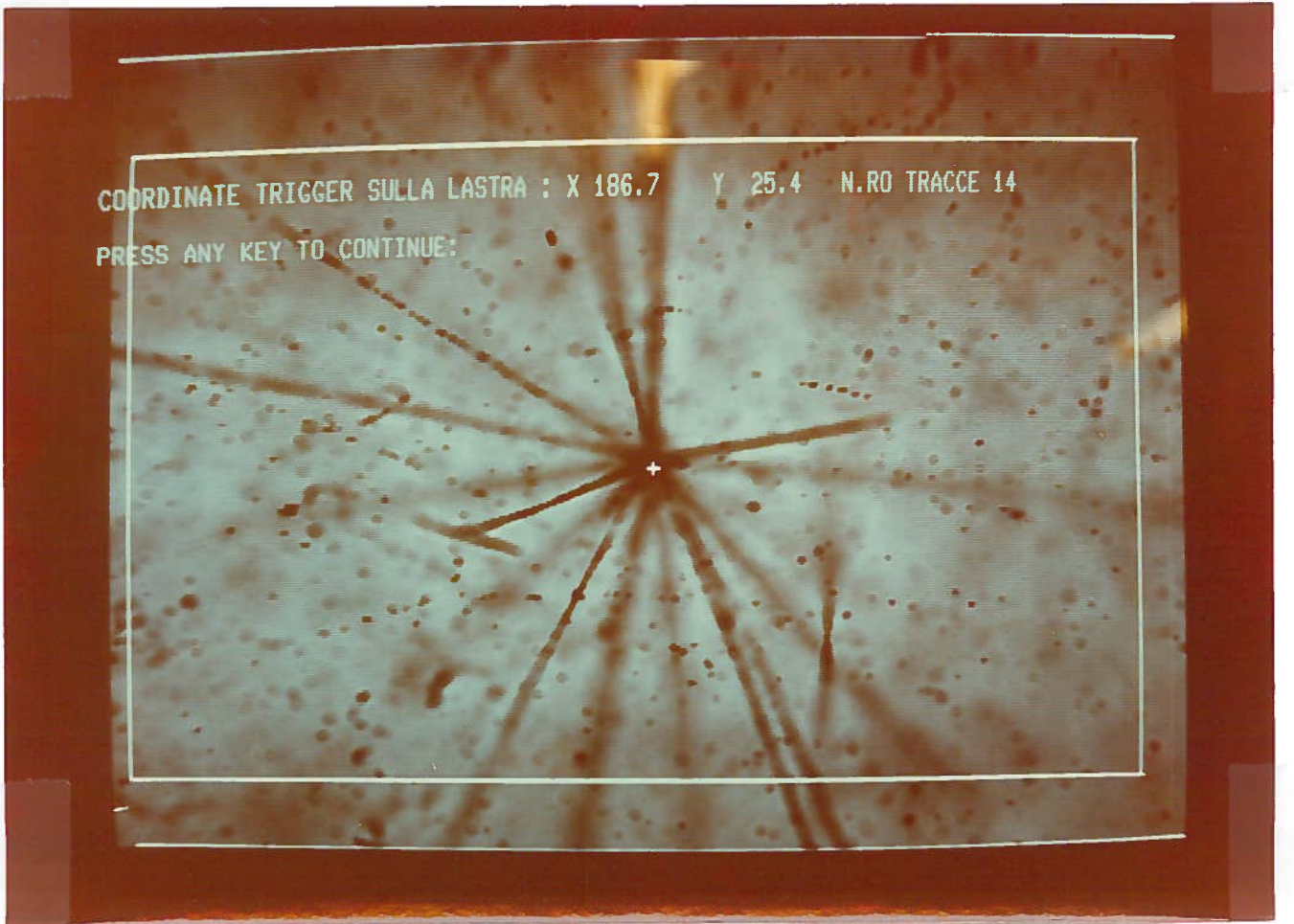
FIG. 2 - (a) The apparatus; (b) An event seen on the screen of the video graphic terminal VT 125.
